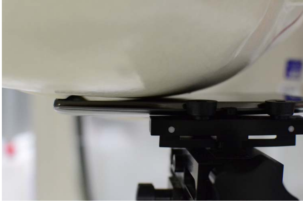
SAR Test Setup Photo 1 – Right Cheek
