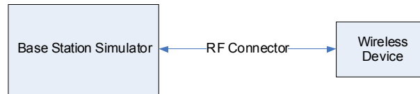
Figure 9-2 Power Measurement Setup
