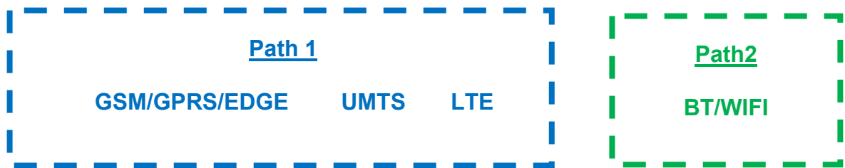
Figure 1-1 Simultaneous Transmission Paths
