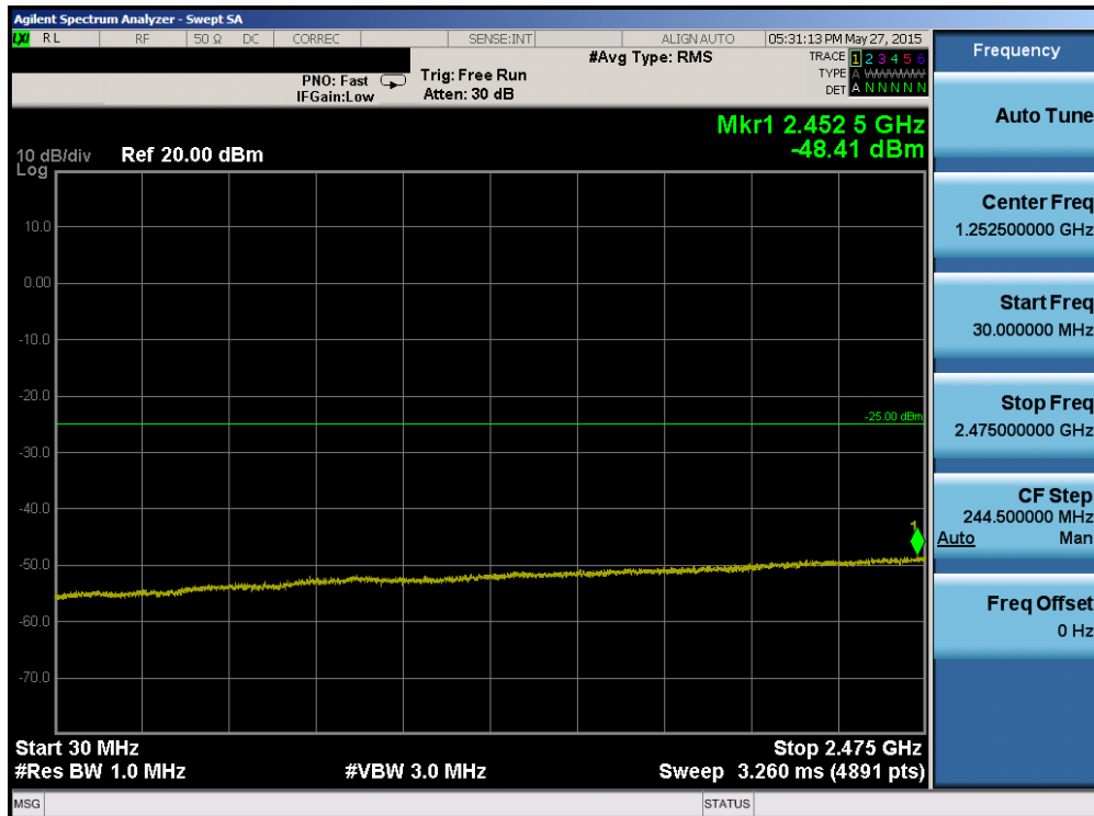
Plot 6-118. Conducted Spurious Plot (Band 7 – 20.0MHz QPSK – RB Size 1, RB Offset 0 – High Channel)
