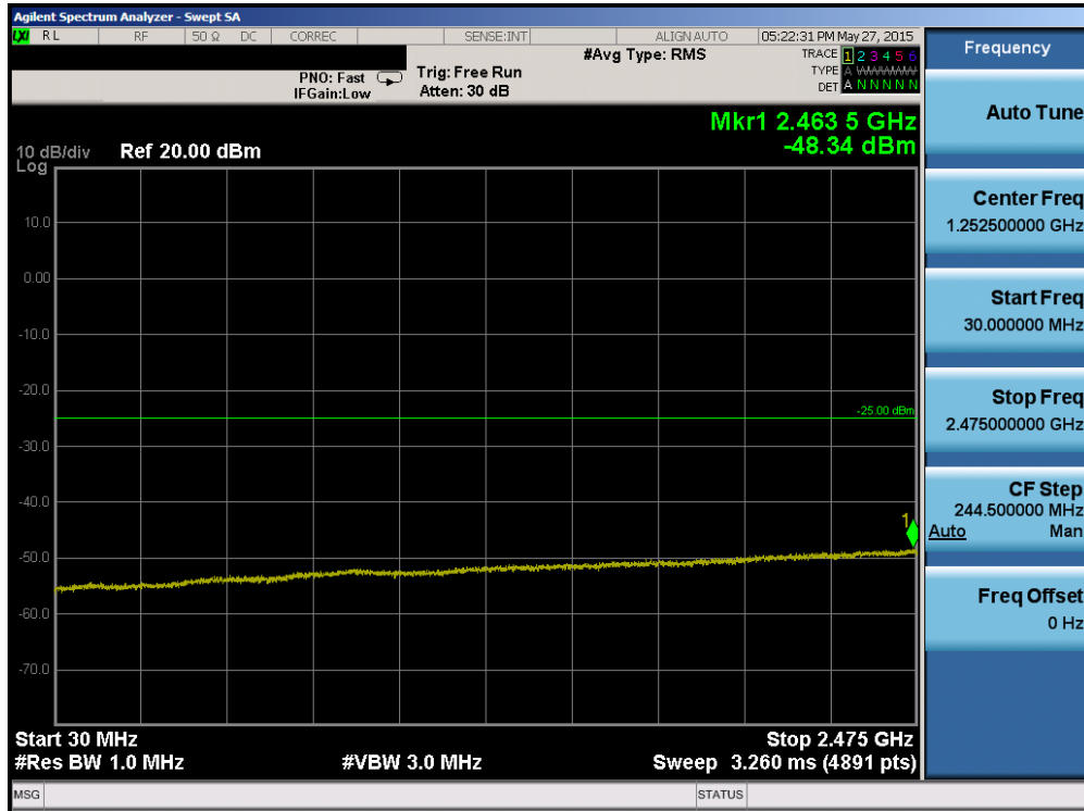
Plot 6-109. Conducted Spurious Plot (Band 7 – 15.0MHz QPSK – RB Size 1, RB Offset 0 – High Channel)
