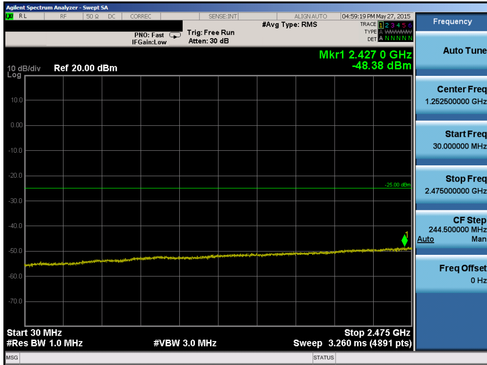
Plot 6-85. Conducted Spurious Plot (Band 7 – 5.0MHz QPSK – RB Size 1, RB Offset 0 – Low Channel)
