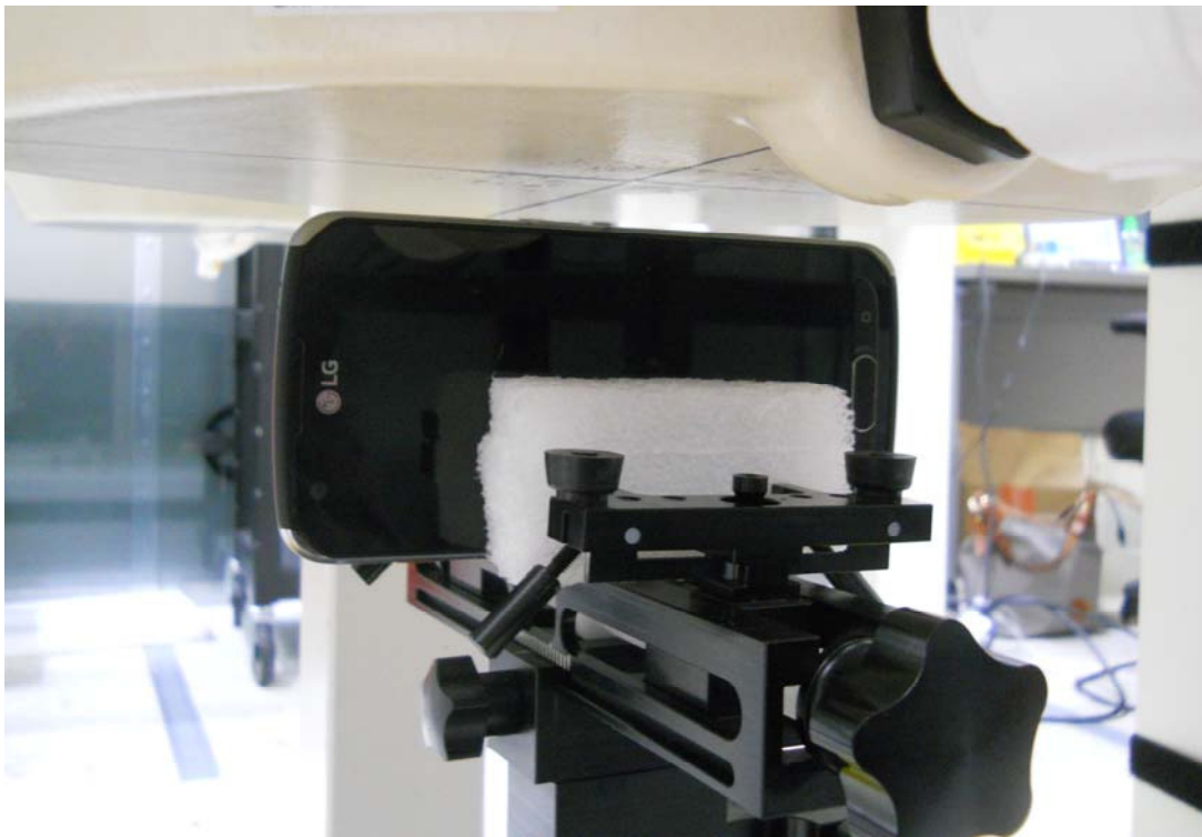
SAR Test Setup Photo 10: Right Edge at 1.0 cm
