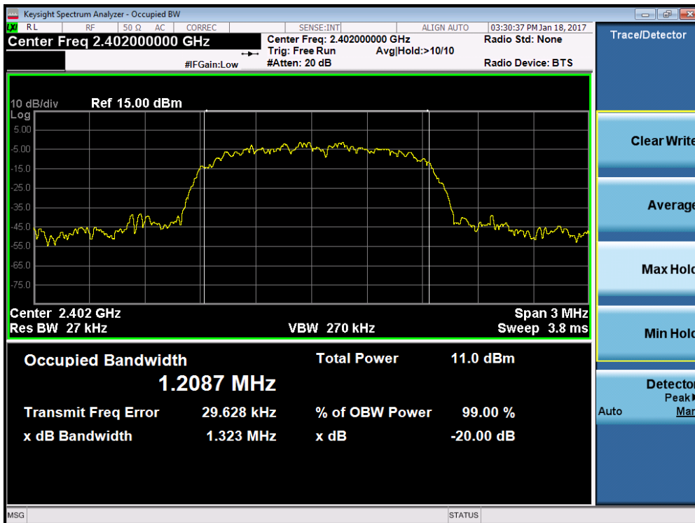
Plot 7-7. 20dB Bandwidth Plot (Bluetooth, 3Mbps – Ch. 0)
