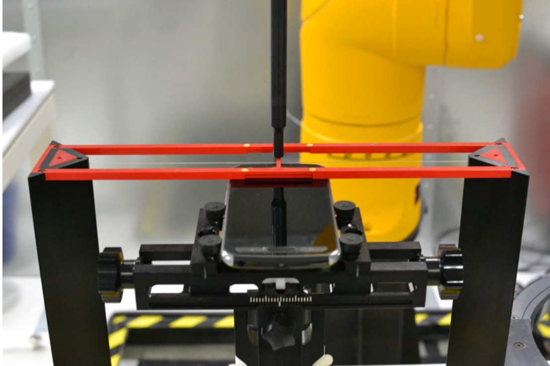
Figure 17-1 Ear Reference Point HAC Phantom Alignment
