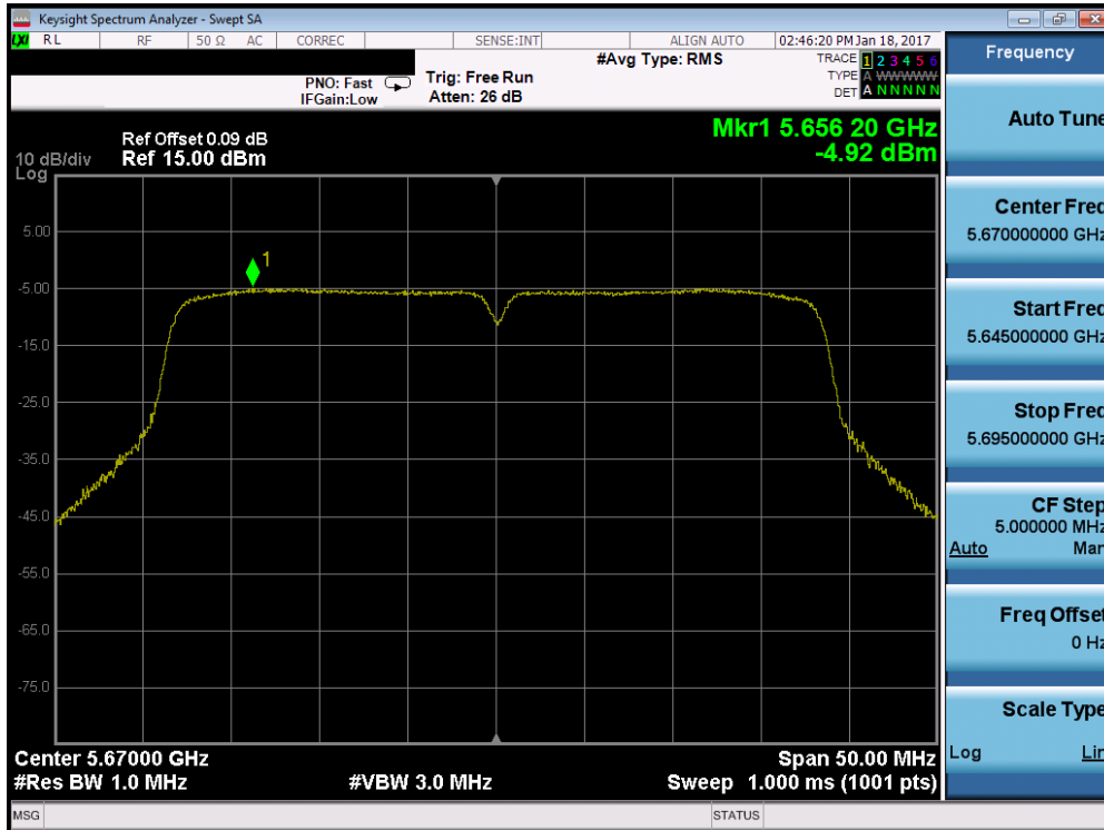
Plot 7-64. Power Spectral Density Plot (40MHz BW 802.11n (UNII Band 2C) – Ch. 134)
