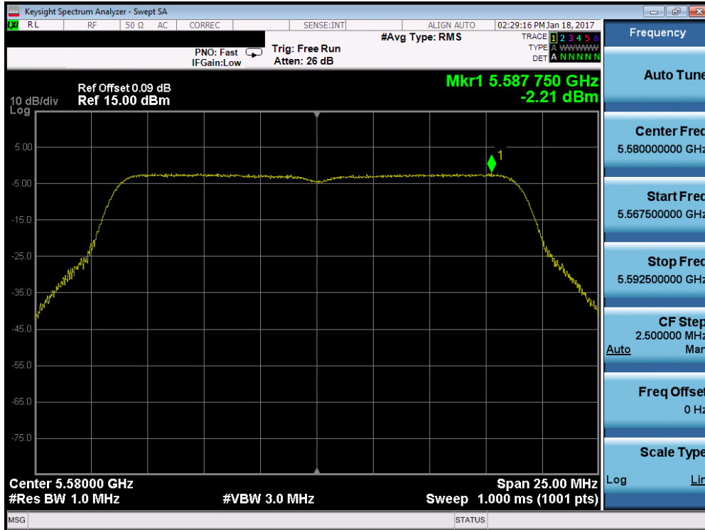
Plot 7-60. Power Spectral Density Plot (20MHz BW 802.11n (UNII Band 2C) – Ch. 116)
