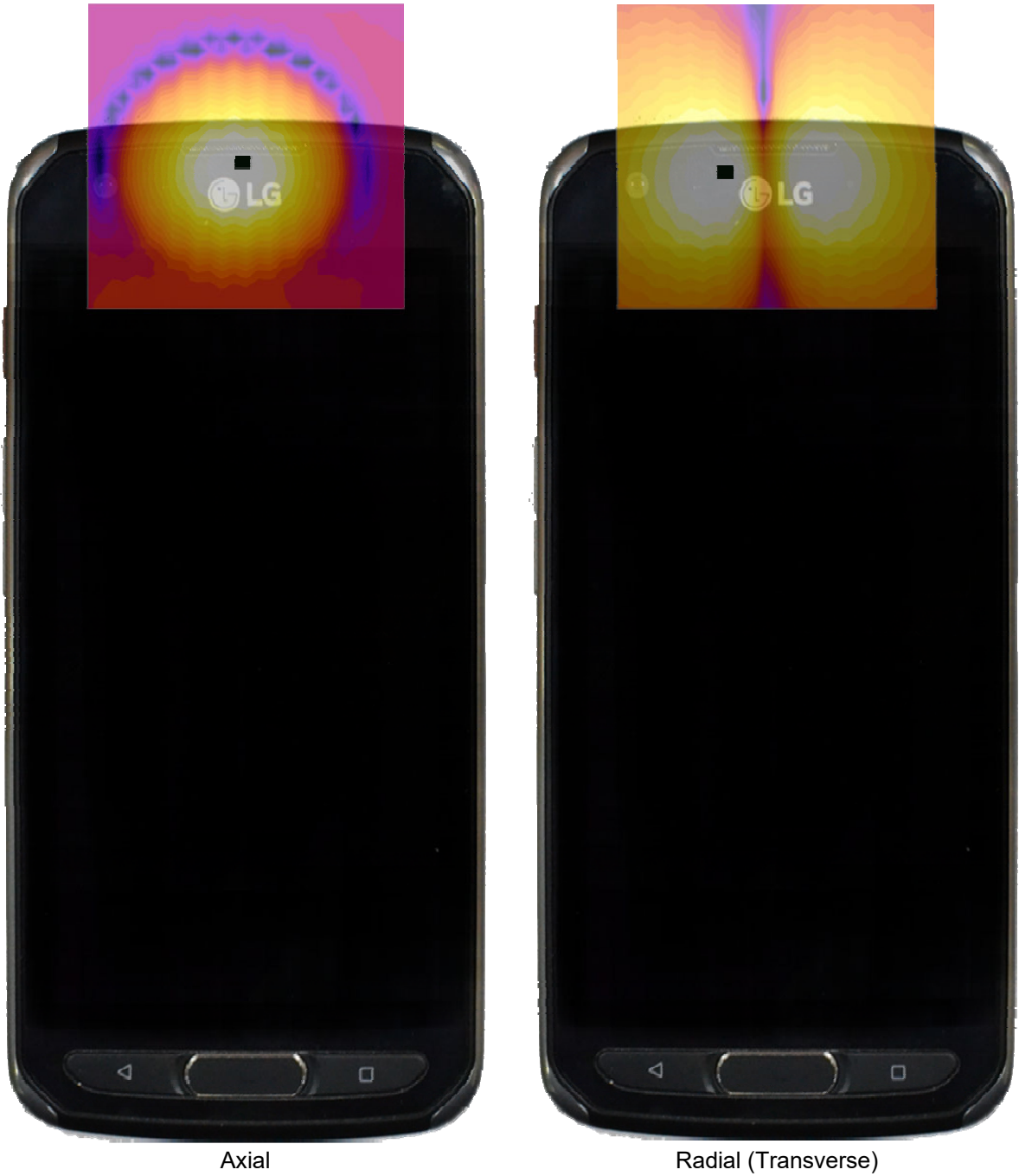
Figure 13-3 T-Coil Scan Overlay Magnetic Field Distributions
