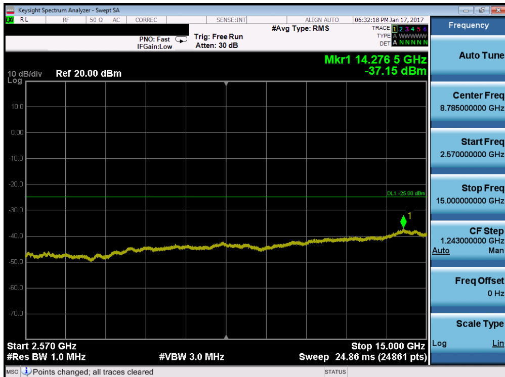
Plot 7-93. Conducted Spurious Plot (Band 7 – 10.0MHz QPSK – RB Size 1, RB Offset 0 – Low Channel)
