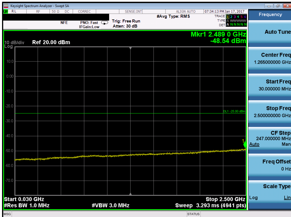
Plot 7-95. Conducted Spurious Plot (Band 7 – 10.0MHz QPSK – RB Size 1, RB Offset 0 – Mid Channel)
