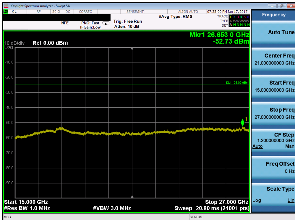
Plot 7-97. Conducted Spurious Plot (Band 7 – 10.0MHz QPSK – RB Size 1, RB Offset 0 – Mid Channel)
