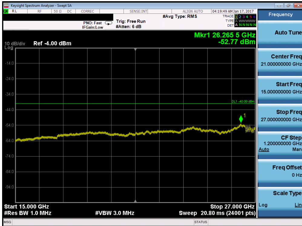
Plot 7-91. Conducted Spurious Plot (Band 30 – 10.0MHz QPSK – RB Size 1, RB Offset 0 – Mid Channel)
