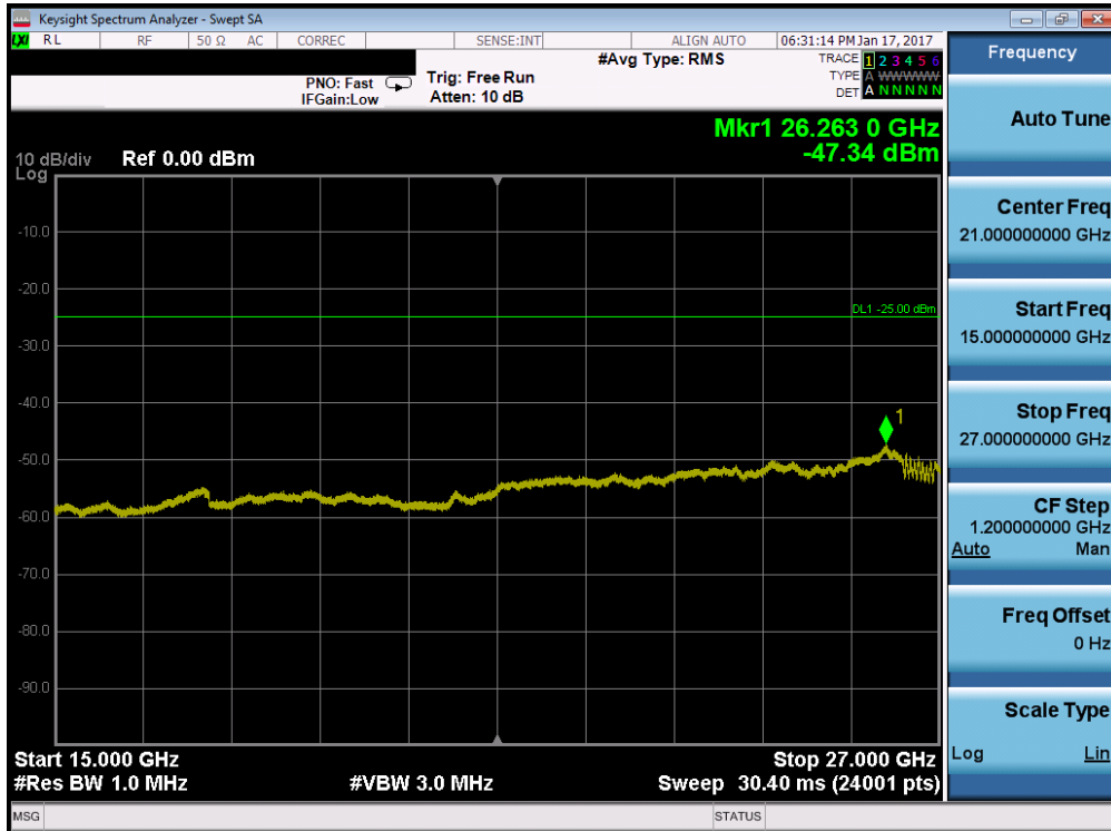
Plot 7-100. Conducted Spurious Plot (Band 7 – 10.0MHz QPSK – RB Size 1, RB Offset 0 – High Channel)
