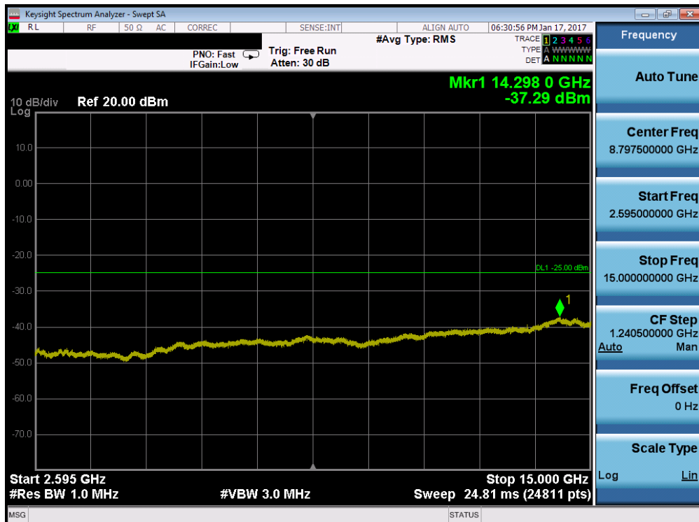
Plot 7-99. Conducted Spurious Plot (Band 7 – 10.0MHz QPSK – RB Size 1, RB Offset 0 – High Channel)
