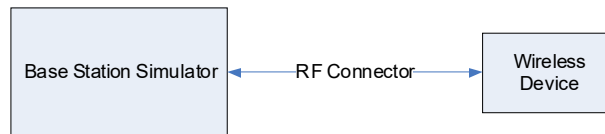
Figure 9-2 Power Measurement Setup
