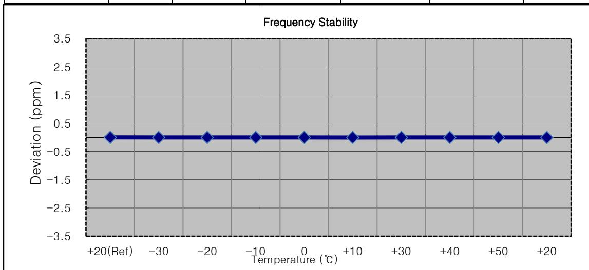
**7.6.4 FREQUENCY STABILITY (20 MHz Band 7 LTE)** OPERATING FREQUENCY: 2,535,000,000 Hz CHANNEL: 21100 (20 MHz) REFERENCE VOLTAGE: 3.8 VDC DEVIATION LIMIT: -
