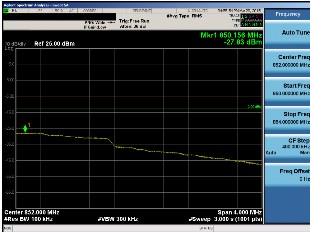
Plot 6-115. Upper Extended Band Edge Plot (Band 5 – Band 5 – 3.0MHz QPSK – RB Size 15)
