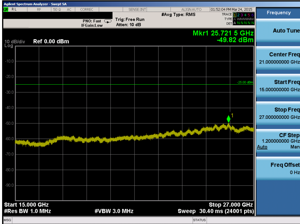
Plot 6-93. Conducted Spurious Plot (Band 7 – 5.0MHz QPSK – RB Size 1, RB Offset 0 – High Channel)
