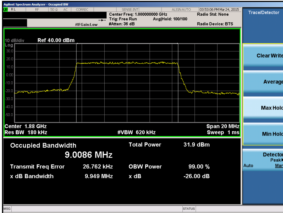
Plot 6-35. Occupied Bandwidth Plot (Band 2 – 10.0MHz QPSK – RB Size 50)
