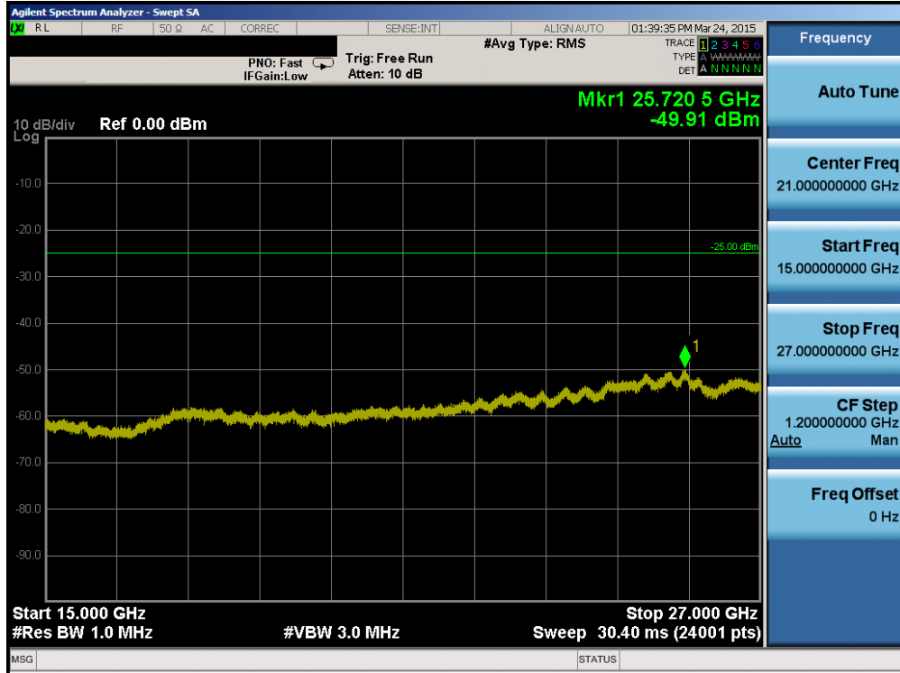
Plot 6-87. Conducted Spurious Plot (Band 7 – 5.0MHz QPSK – RB Size 1, RB Offset 0 – Low Channel)
