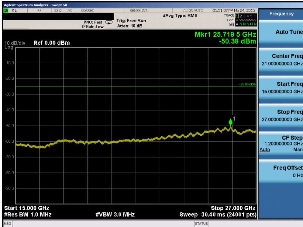
Plot 6-90. Conducted Spurious Plot (Band 7 – 5.0MHz QPSK – RB Size 1, RB Offset 0 – Mid Channel)
