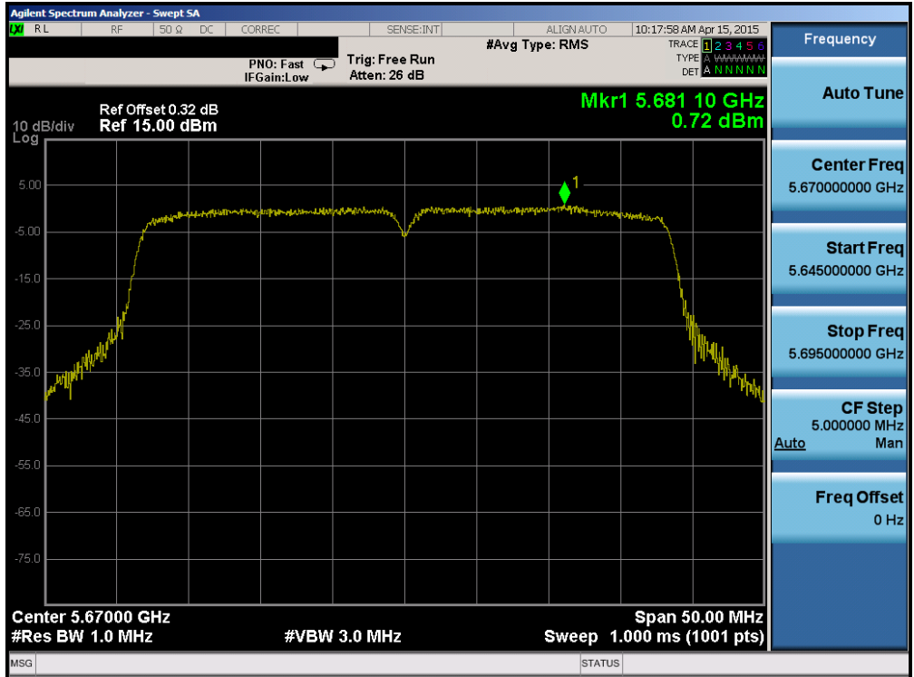
Plot 6-58. Power Spectral Density Plot (40MHz BW 802.11n (UNII Band 2C) – Ch. 134)
