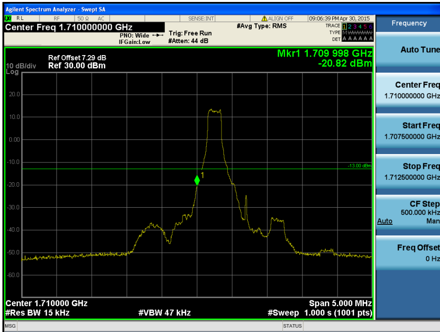
LTE Band 4 / 1.4MHz / 16QAM - RB Size/Offset (1/0)
