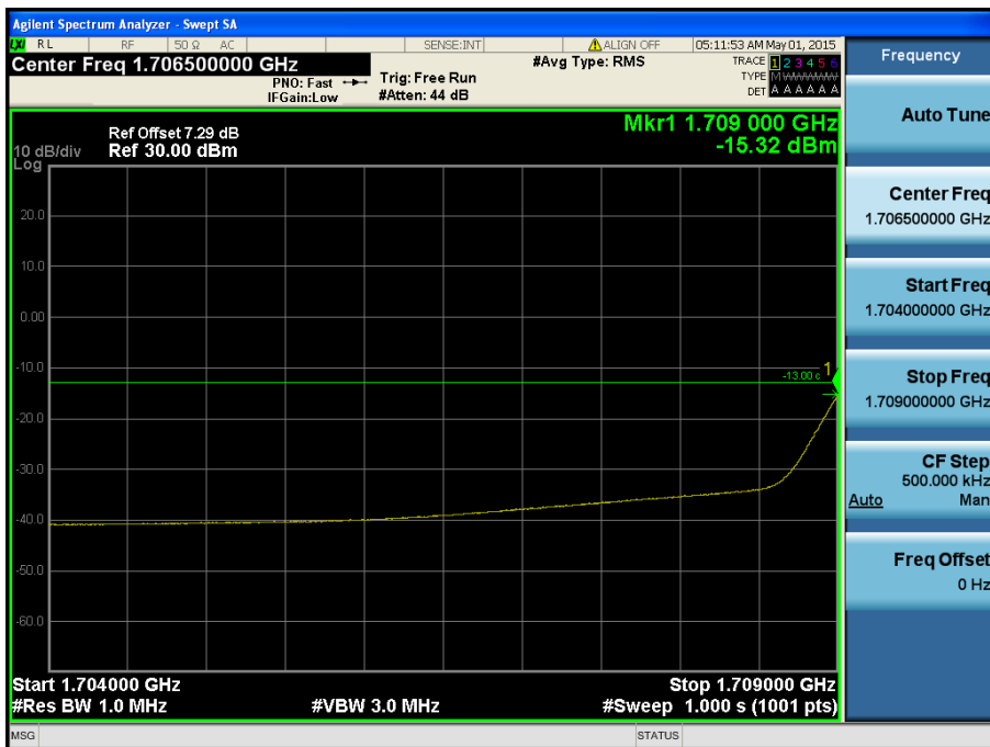
LTE Band 4 / 1.4MHz / QPSK - RB Size/Offset (3/2)
