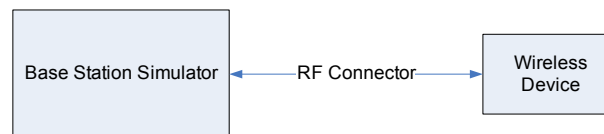
Figure 9-2 Power Measurement Setup
