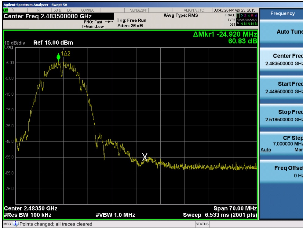
Plot 6-22. Band Edge Plot (802.11g – Ch. 11)
