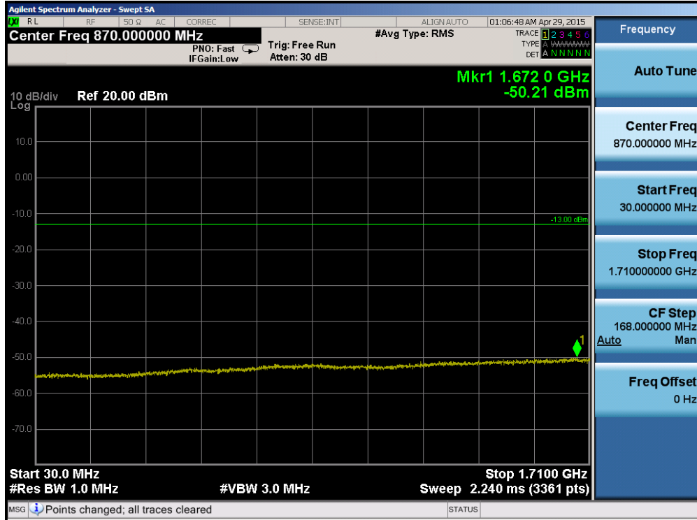
Plot 6-61. Conducted Spurious Plot (Band 4 – 5.0MHz QPSK – RB Size 1, RB Offset 0 – High Channel)
