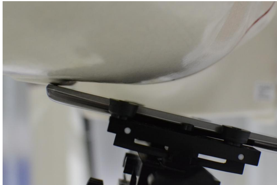
SAR Test Setup Photo 2 – Right Tilt
