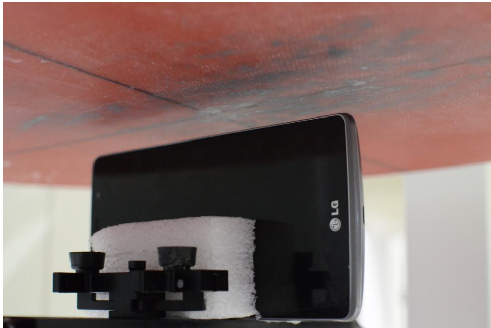
SAR Test Setup Photo 18 – Right Edge at 1.0 cm
