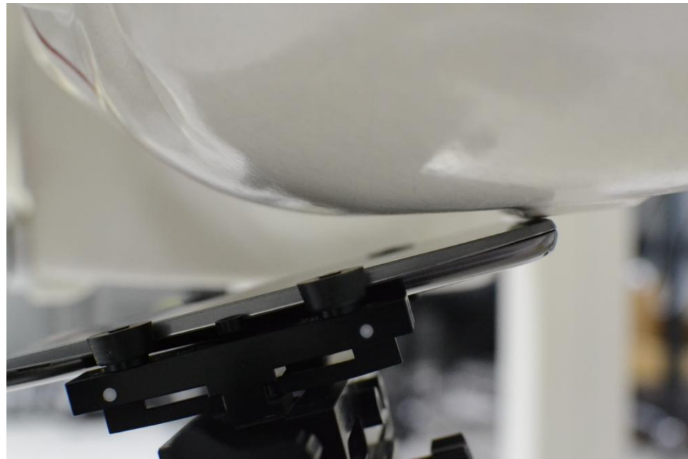
SAR Test Setup Photo 6 – Left Tilt
