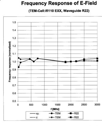
Figure 4-2 E-Field Probe Frequency Response
