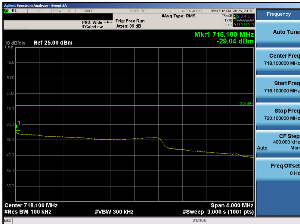
Plot 6-67. Upper Extended Band Edge Plot (Band 12 – 3.0MHz QPSK – RB Size 15)
