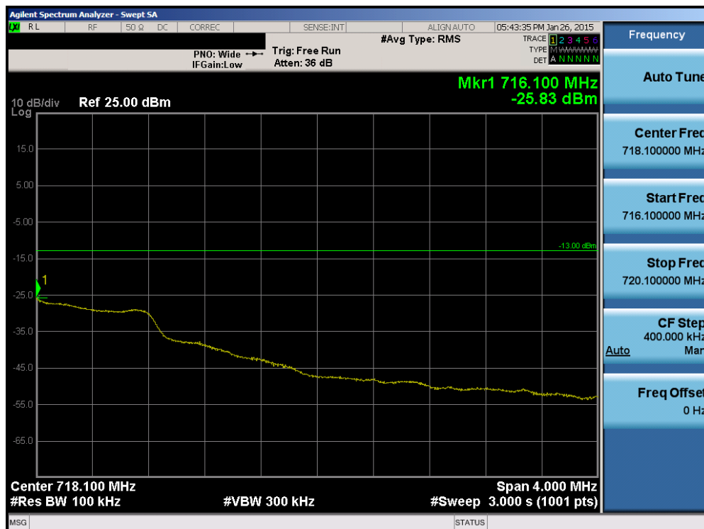
Plot 6-63. Upper Extended Band Edge Plot (Band 12 - 1.4MHz QPSK - RB Size 6)
