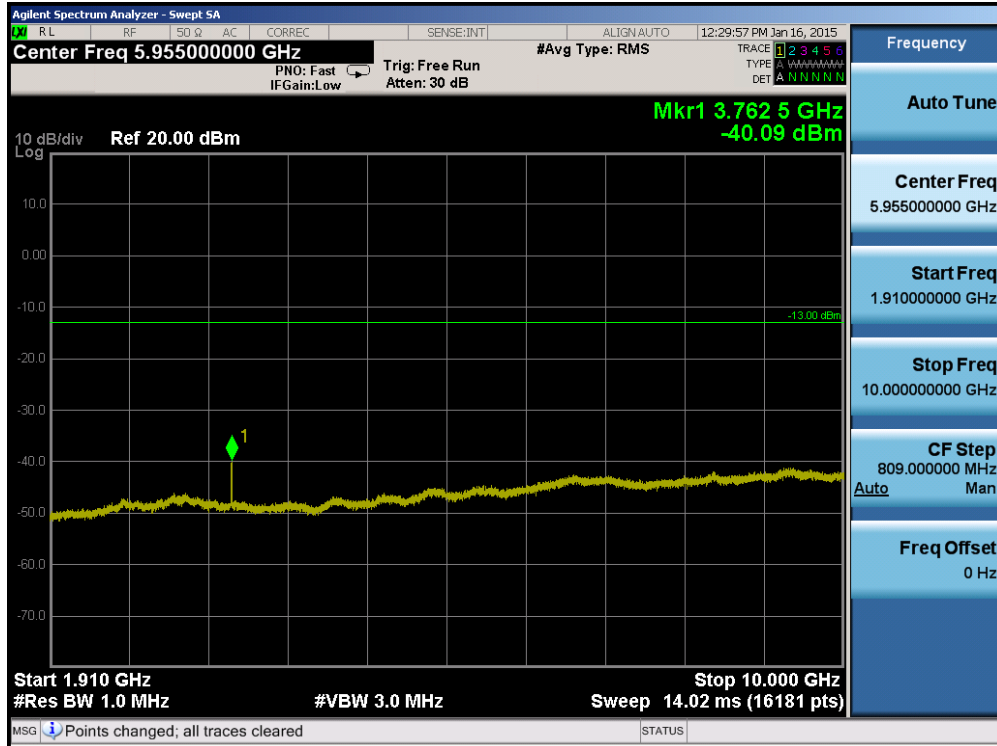
Plot 6-48. Conducted Spurious Plot (PCS WCDMA Mode – Ch. 9400)
