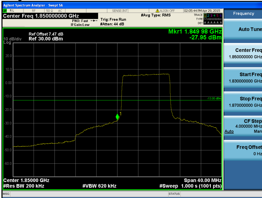
LTE Band 2 / 20MHz / QPSK - RB Size/Offset (50/0)
