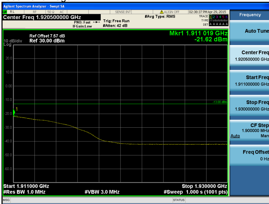
LTE Band 2 / 20MHz / QPSK - RB Size/Offset (50/50)
