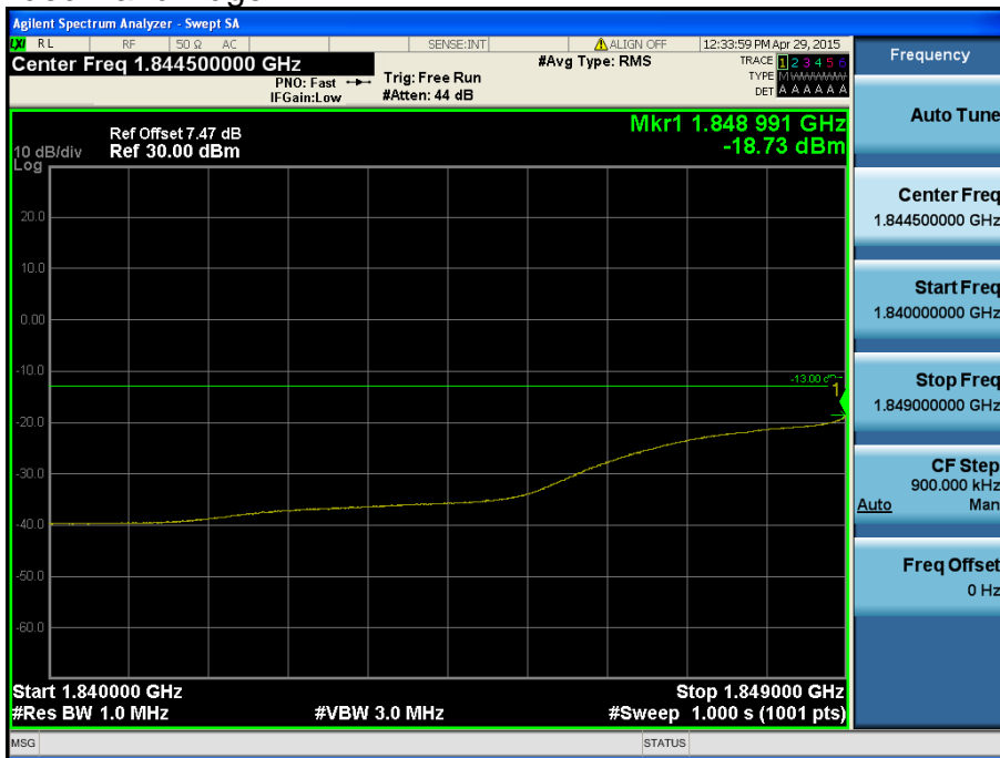
LTE Band 2 / 10MHz / QPSK - RB Size/Offset (25/0)
