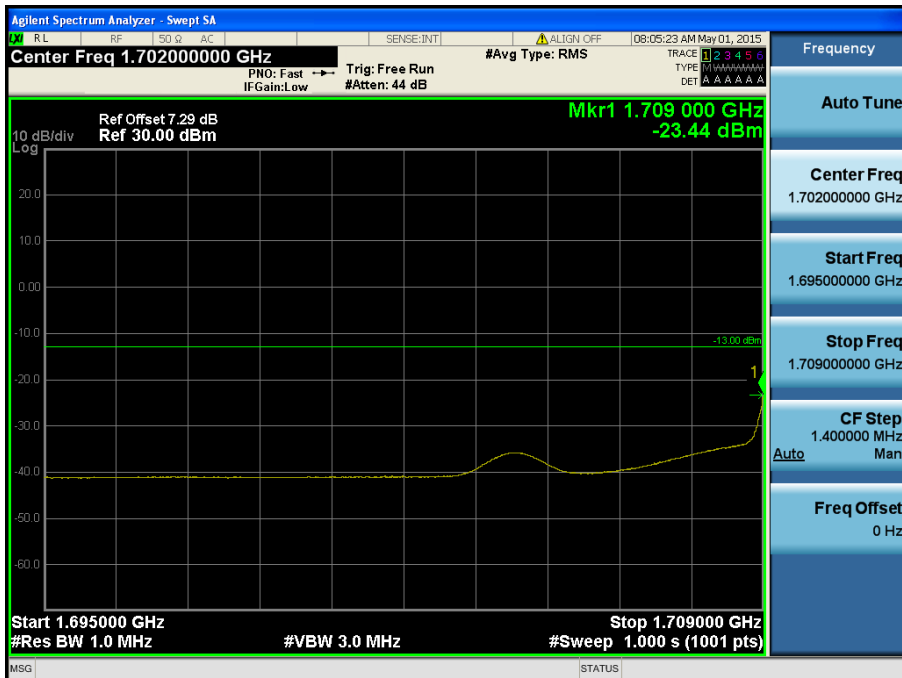
LTE Band 4 / 15MHz / QPSK - RB Size/Offset (1/0)
