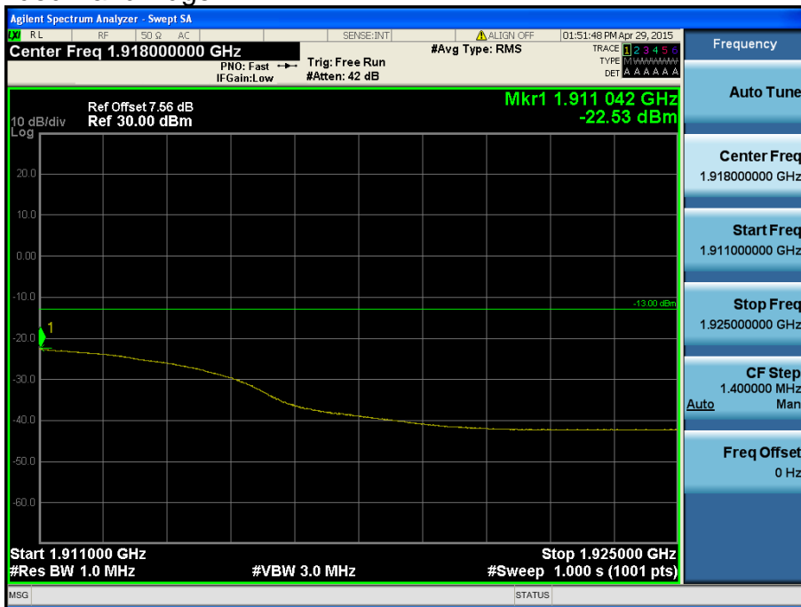
LTE Band 2 / 15MHz / QPSK - RB Size/Offset (36/37)
