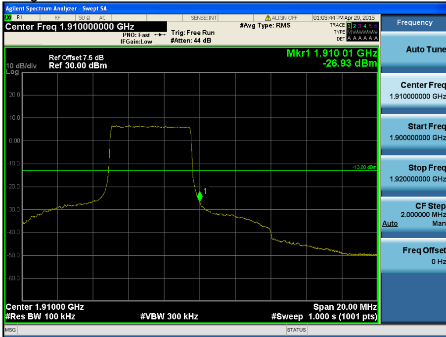
LTE Band 2 / 10MHz / QPSK - RB Size/Offset (25/25)
