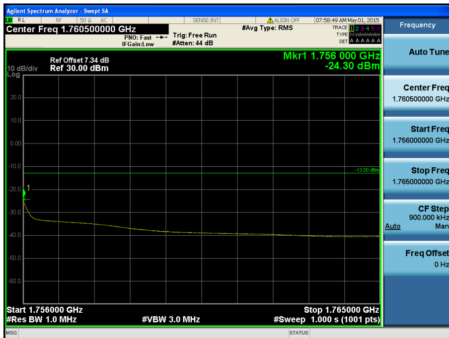
LTE Band 4 / 10MHz / QPSK - RB Size/Offset (25/25)
