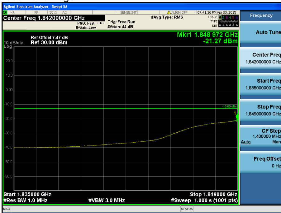
LTE Band 2 / 15MHz / 16QAM - RB Size/Offset (36/0)
