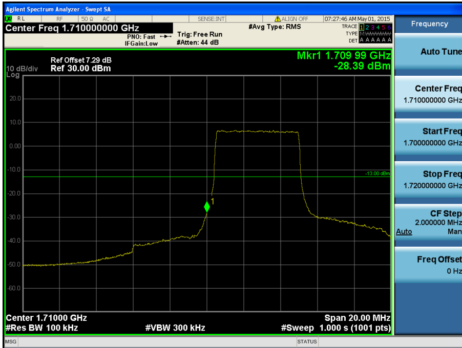
LTE Band 4 / 10MHz / QPSK - RB Size/Offset (25/0)
