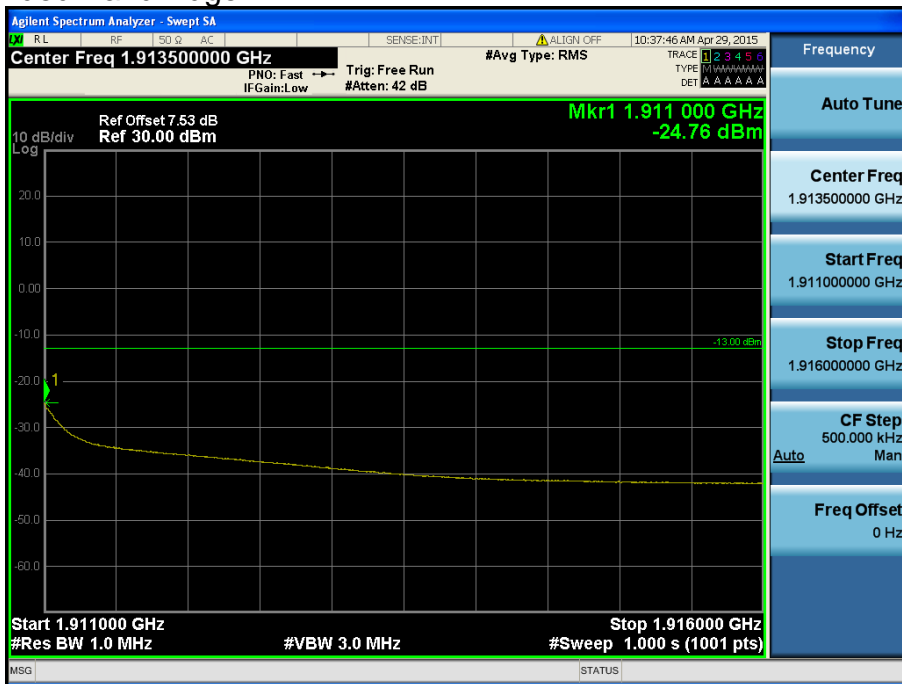
LTE Band 2 / 1.4MHz / QPSK - RB Size/Offset (3/0)
