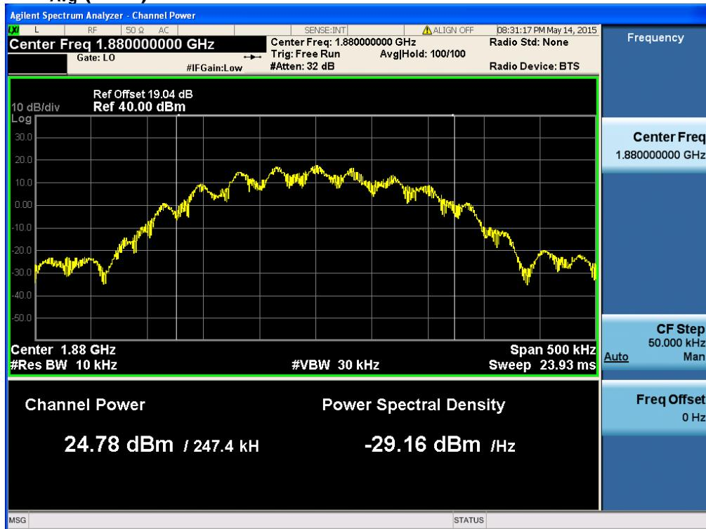
$$\text{PAR (dB)} = \mathbf{P}_{\text{Pk}} \text{ (dBm)} - \mathbf{P}_{\text{Avg}} \text{ (dBm)} = 28.51 \text{ dBm} - 24.78 \text{ dBm} = 3.73 \text{ dB}$$
