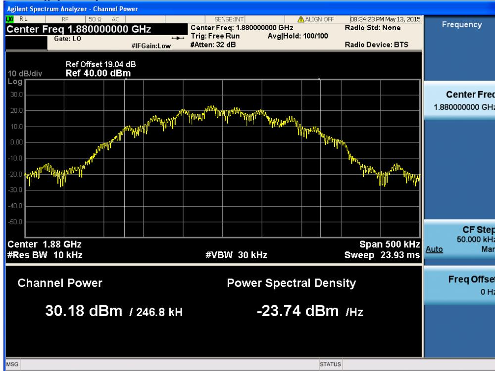
$$\text{PAPR (dB)} = P_{Pk} (\text{dBm}) - P_{Avg} (\text{dBm}) = 30.70 \text{ dBm} - 30.18 \text{ dBm} = 0.52 \text{ dB}$$
