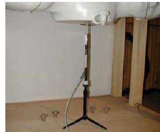
Figure 11.1 Dipole Verification Test Setup Diagram & Photo
