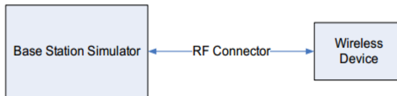
Figure 10.2 Power Measurement Setup
