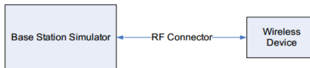
Figure 10.1 Power Measurement Setup
