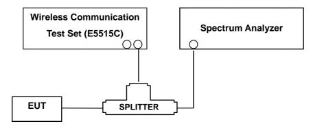
(Configuration of conducted Emission measurement)
