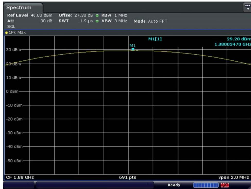
■ GSM1900 MODE (661 CH.) Peak-to-Average Ratio P<sub>Avg</sub>
