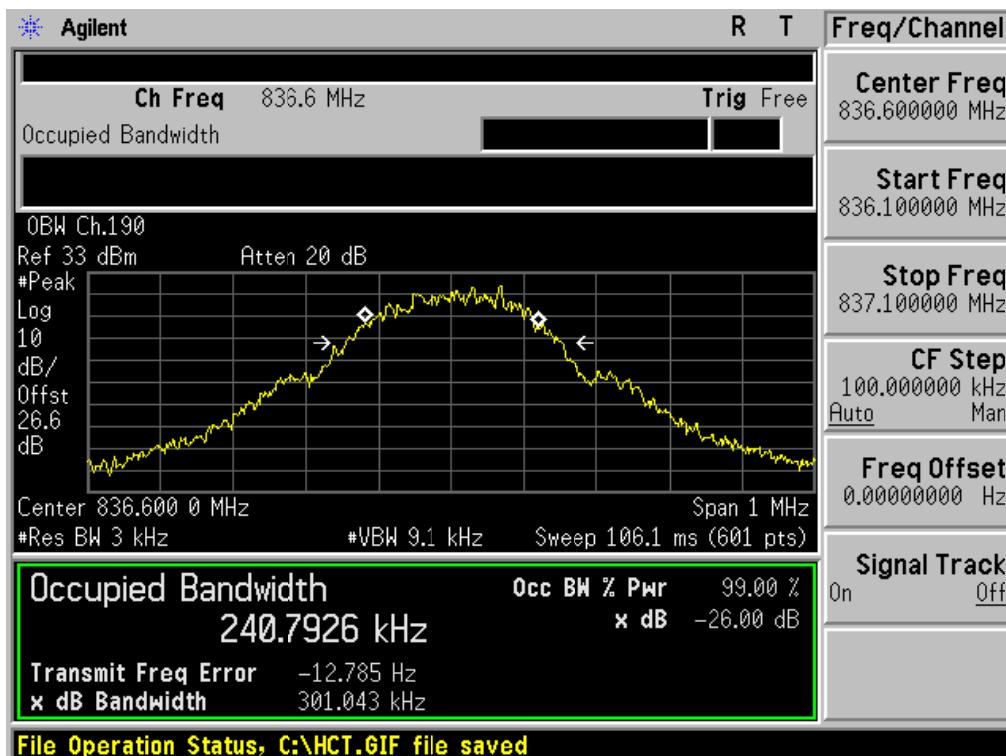
■ GSM850 MODE (251 CH.) Occupied Bandwidth
