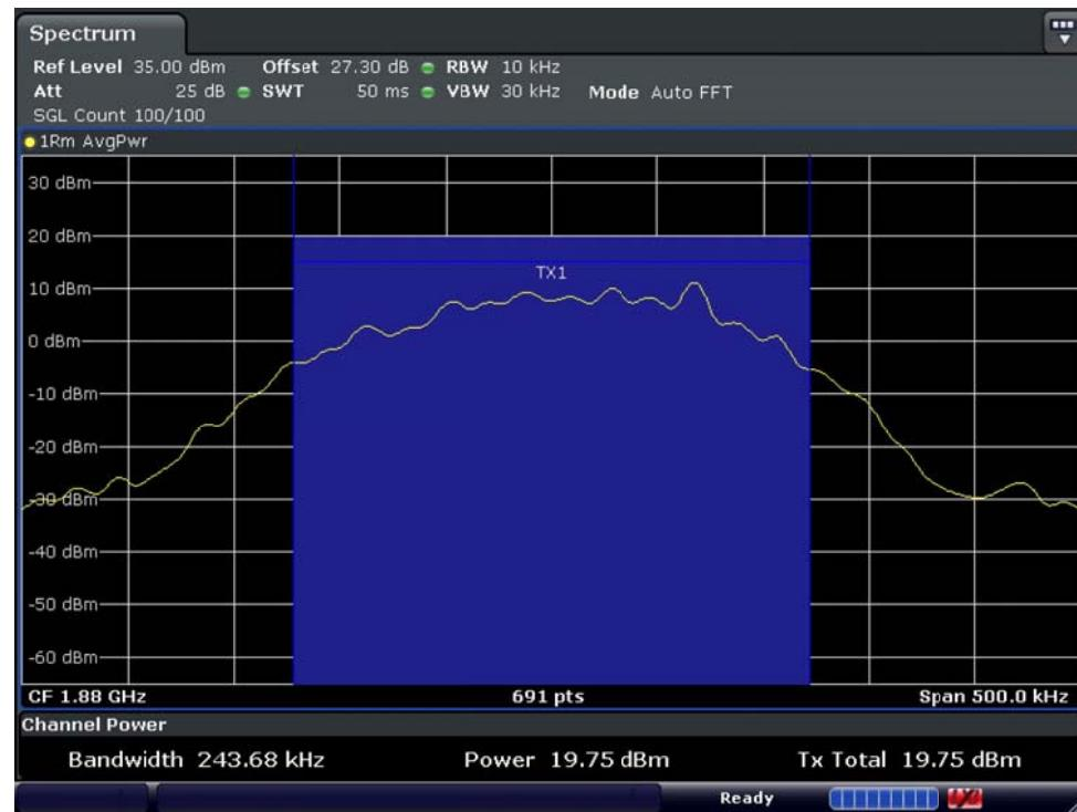
■ GSM1900 MODE (661 CH.) Peak-to-Average Ratio P<sub>Avg</sub>
