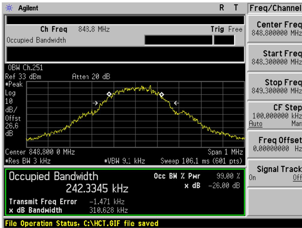
■ GSM850 EDGE (128 CH.) Occupied Bandwidth
