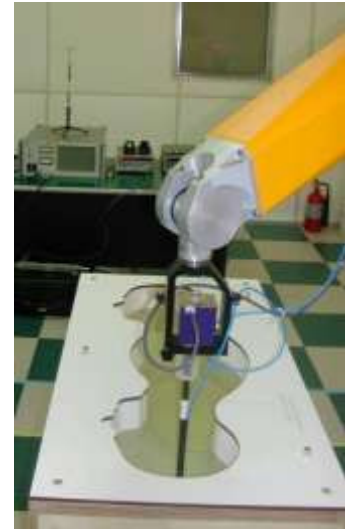
Figure 3. Photograph of the probe and the Phantom
