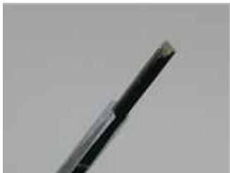
Figure 6. EX3DV4 E-field Probe
