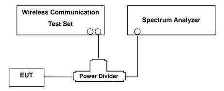
(Configuration of conducted Emission measurement)
