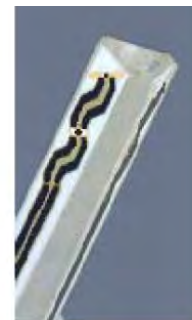
Figure F.2.2 Probe Thick-Film Technique
