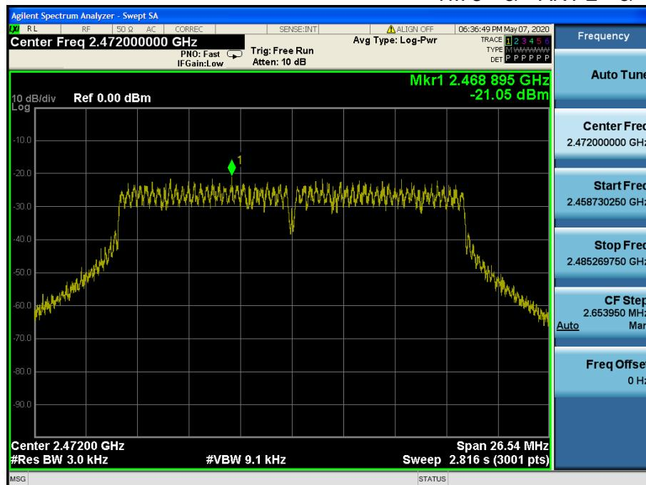
**8.4 Out of band emissions at the band edge / conducted spurious emissions****■ Test requirements and limit, §15.247(d)**
