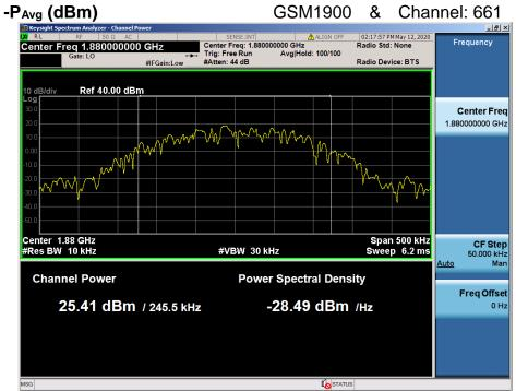
PAPR (dB) =  $P_{Pk}$  (dBm) -  $P_{Avg}$  (dBm) = 25.94 dBm - 25.41 dBm = 0.53 dB
