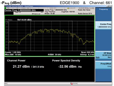
PAPR (dB) =  $P_{Pk}$  (dBm) -  $P_{Avg}$  (dBm) = 24.91 dBm - 21.27 dBm = 3.64 dB
