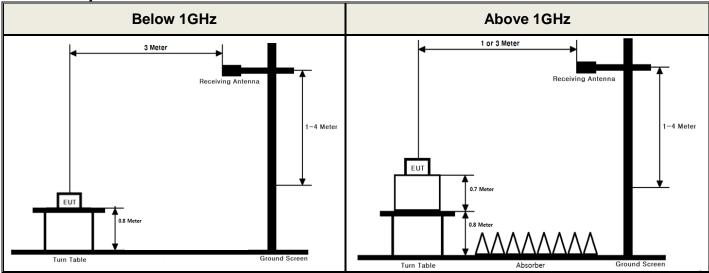
These measurements were performed at 3 m test site. The equipment under test is placed on a non-conductive table 1.5 meters above a turntable which is flush with the ground plane and 3 meters from the receive antenna. For measurements above 1 GHz absorbers are placed on the floor between the turn table and the antenna mast in such a way so as to maximize the reduction of reflections. For measurements below 1 GHz, the absorbers are removed.
