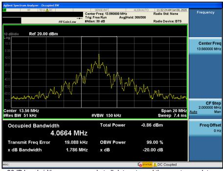
Note1: The 20dB bandwidth was measured at all data rate and the worst case data was reported (This test item was tested at 212 kbps.)
