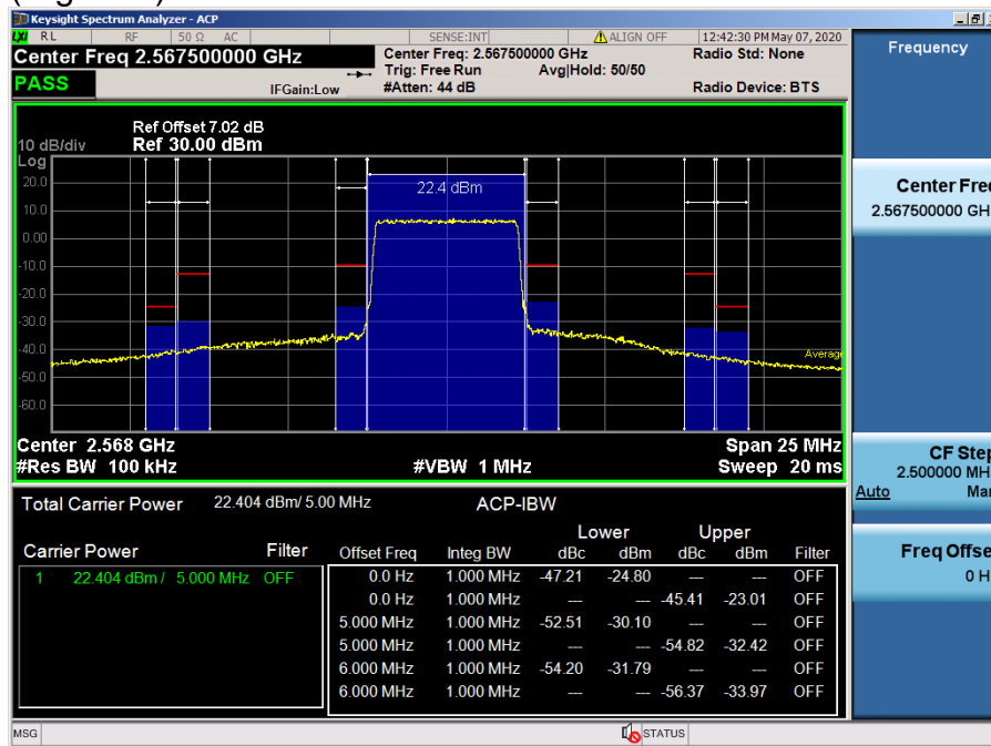
LTE Band 7 / 5 MHz / 16QAM - RB Size/Offset (25/0)
