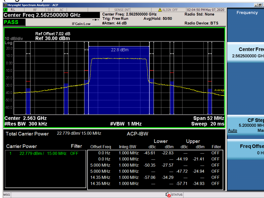
LTE Band 7 / 15 MHz / 16QAM - RB Size/Offset (75/0)
