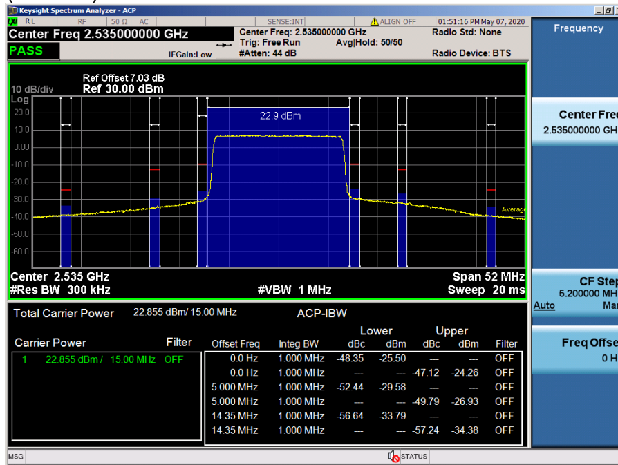
LTE Band 7 / 15 MHz / 16QAM - RB Size/Offset (75/0)
