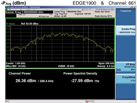
PAPR (dB) =  $P_{Pk}$  (dBm) -  $P_{Avg}$  (dBm) = 27.03 dBm - 26.36 dBm = 0.67 dB
