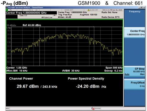
PAPR (dB) =  $P_{Pk}$  (dBm) -  $P_{Avg}$  (dBm) = 30.24 dBm - 29.67 dBm = 0.57 dB
