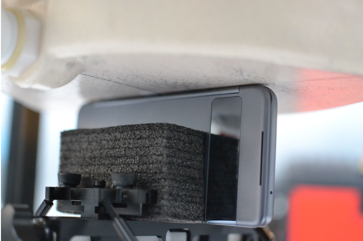
SAR Test Setup Photo 41 – Left Edge with Dual Display Accessory Position #1 at 0 mm
