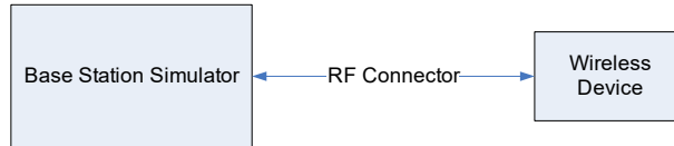
Figure 9-2 Power Measurement Setup
