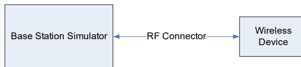
Figure 9-3 Power Measurement Setup
