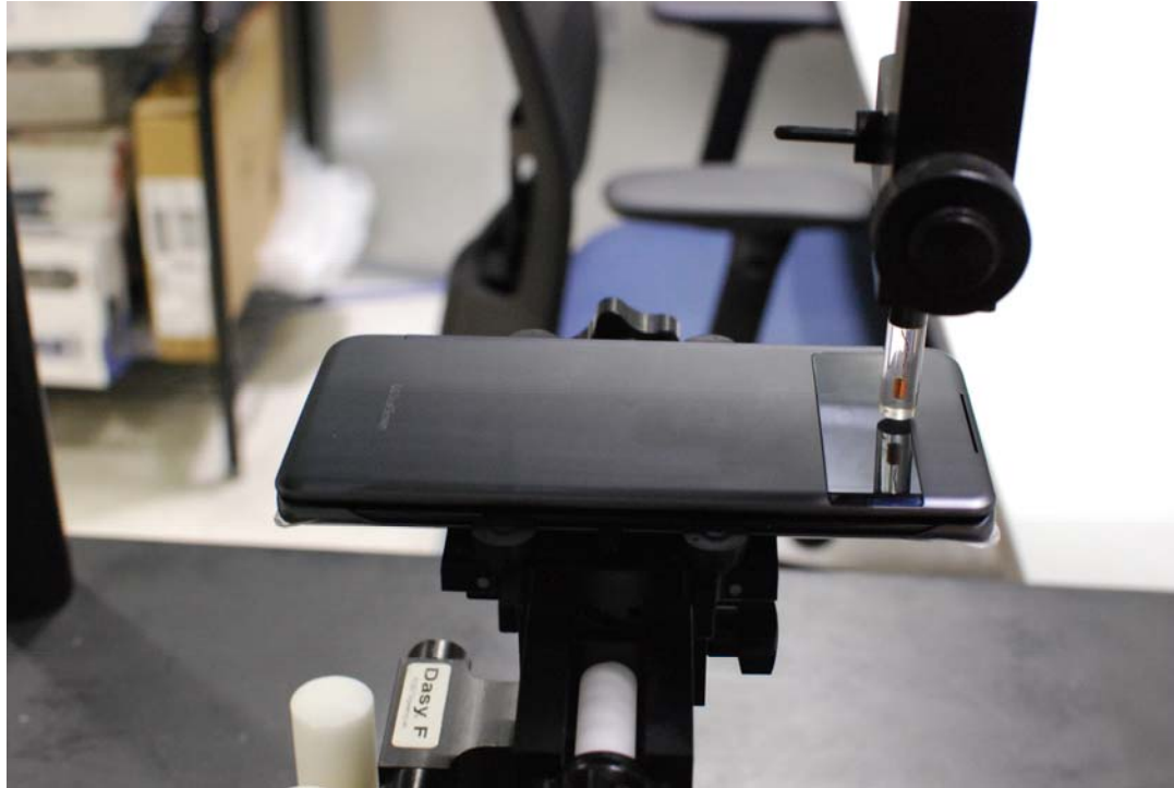
Figure 16-3 Test Setup for Wireless Device – Dual Display Closed
