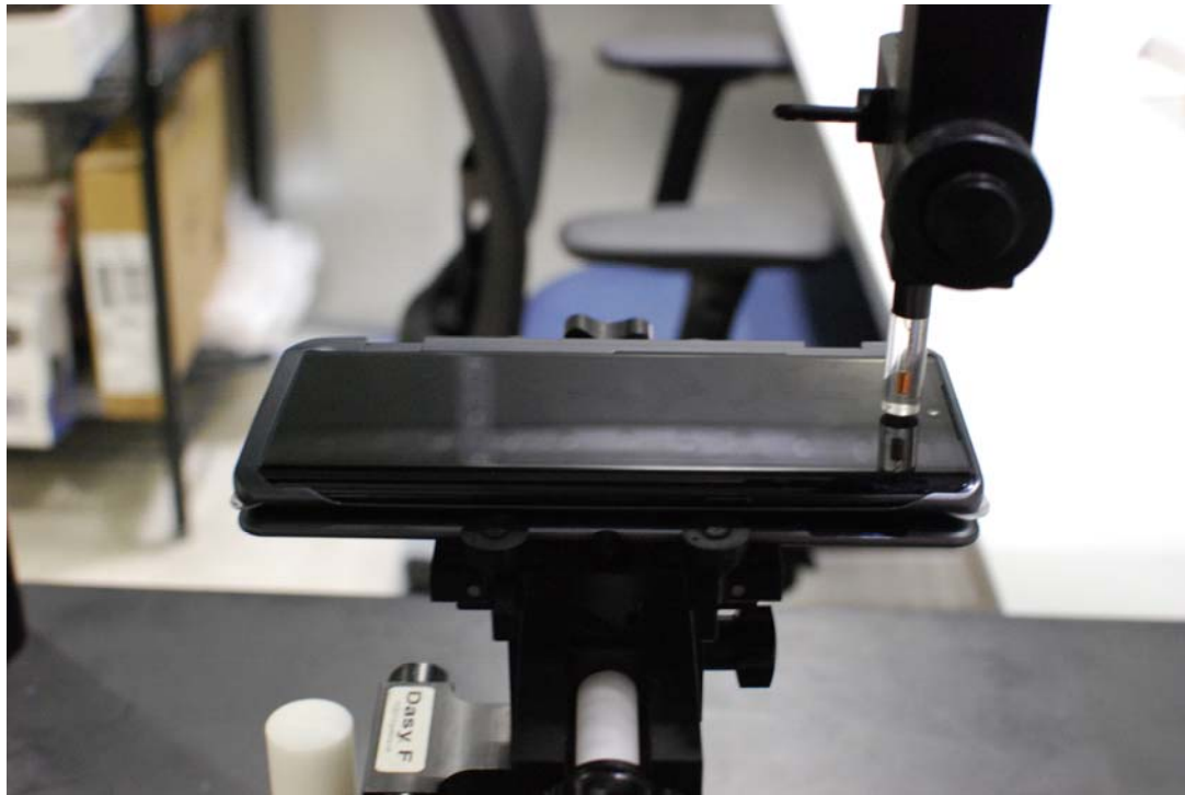
Figure 16-5 Test Setup for Wireless Device – Dual Display Open
