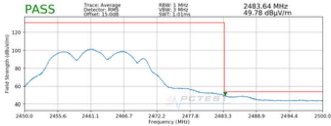
Plot 7-13. Radiated Restricted Upper Band Edge Measurement MIMO (Average) (w/ Dual Display)
