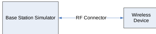
Figure 9-2 Power Measurement Setup
