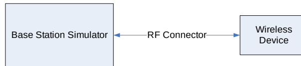
Figure 9-4 Power Measurement Setup
