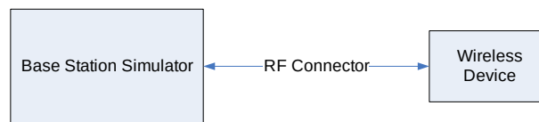
Figure 9-3 Power Measurement Setup
