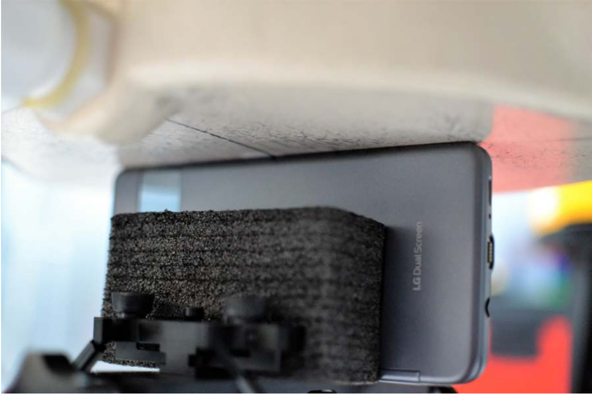
SAR Test Setup Photo 33 – Right Edge with Dual Display Accessory Position #1 at 0 mm
