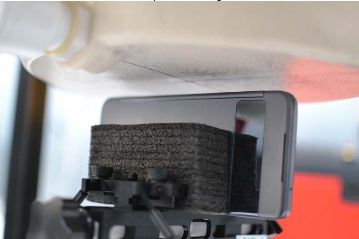
SAR Test Setup Photo 36 – Left Edge with Dual Display Accessory Position #1 at 10 mm
