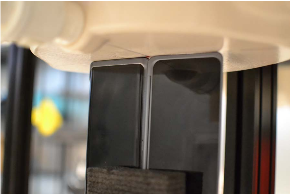
SAR Test Setup Photo 26 – Bottom Edge with Dual Display Accessory Position #2 at 0 mm
