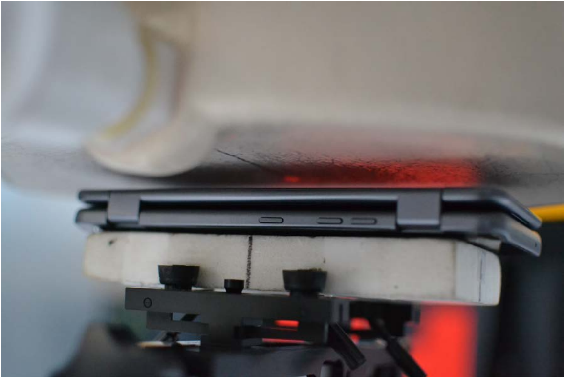
SAR Test Setup Photo 12 – Back Side with Dual Display Accessory Position #3 at 10 mm
