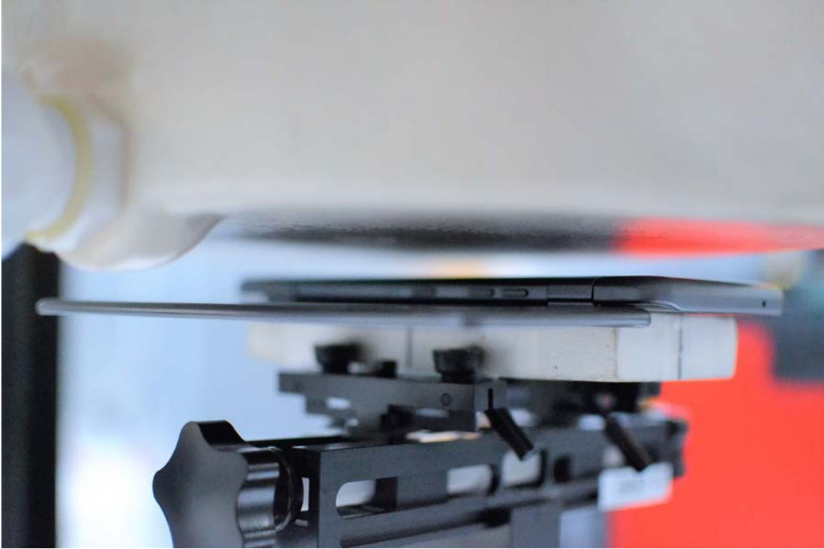
SAR Test Setup Photo 11 – Back Side with Dual Display Accessory Position #2 at 10 mm
