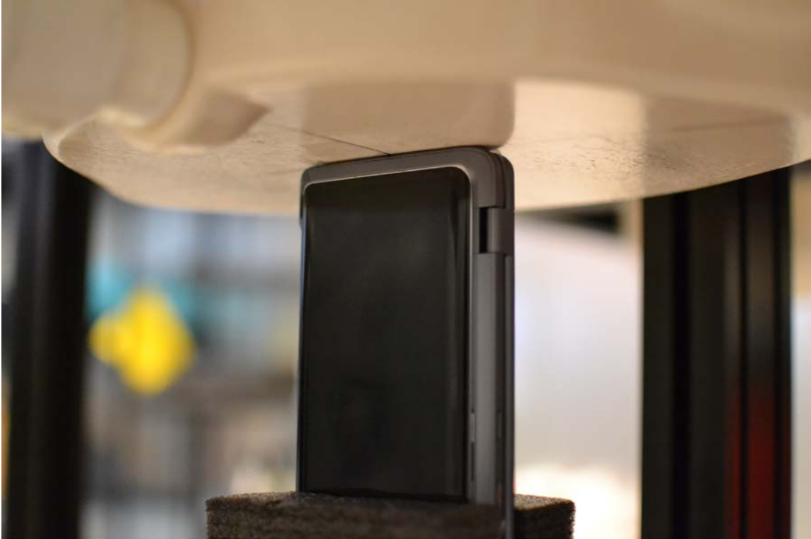
SAR Test Setup Photo 27 – Bottom Edge with Dual Display Accessory Position #3 at 0 mm
