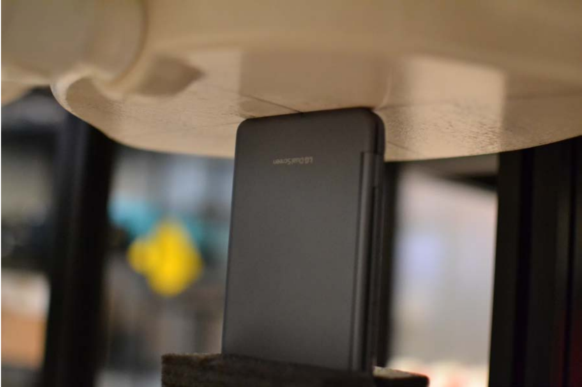
SAR Test Setup Photo 25 – Bottom Edge with Dual Display Accessory Position #1 at 0 mm
