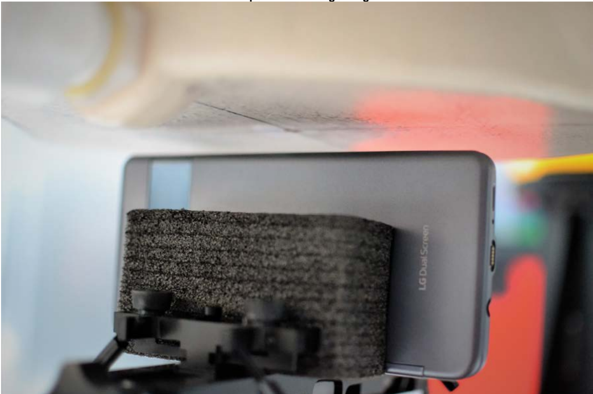
SAR Test Setup Photo 32 – Right Edge with Dual Display Accessory Position #1 at 10 mm
