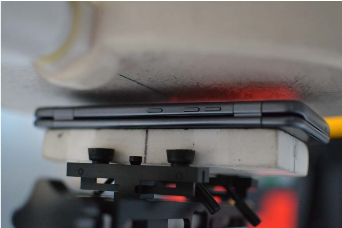
SAR Test Setup Photo 10 – Back Side with Dual Display Accessory Position #1 at 10 mm
