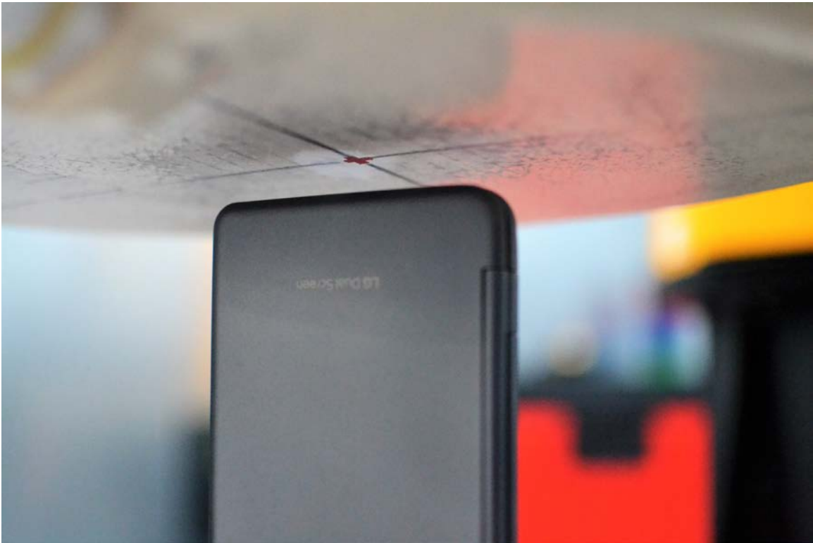
SAR Test Setup Photo 24 – Bottom Edge with Dual Display Accessory Position #1 at 10 mm
