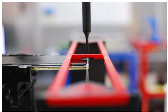
Figure 18-2 HAC Phantom Plane Alignment
