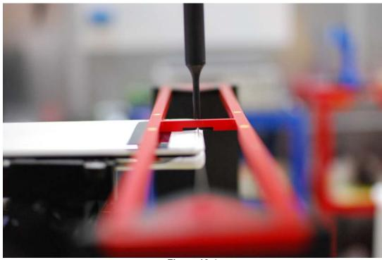
Figure 18-4 HAC Phantom Plane Alignment – Dual Display Closed
