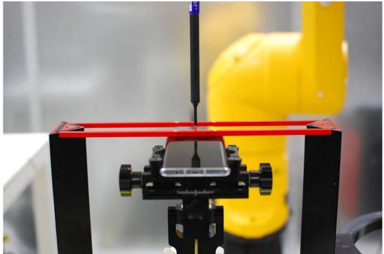
Figure 18-1 Ear Reference Point HAC Phantom Alignment
