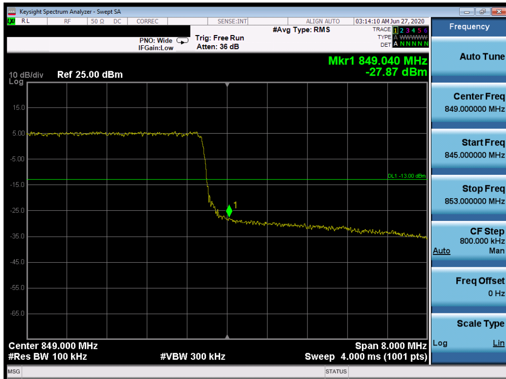
Plot 7-409. Upper Band Edge Plot (Band 26/5 - 10.0MHz QPSK - Full RB Configuration)
