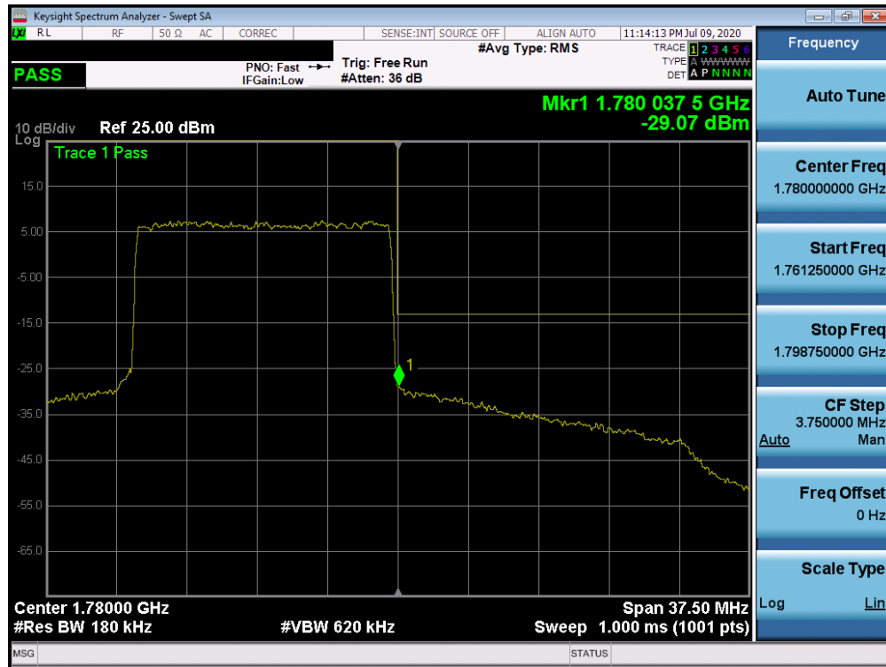
Plot 7-458. Upper Band Edge Plot (n66 - 15MHz DFT-s-OFDM-QPSK - Full RB Configuration)
