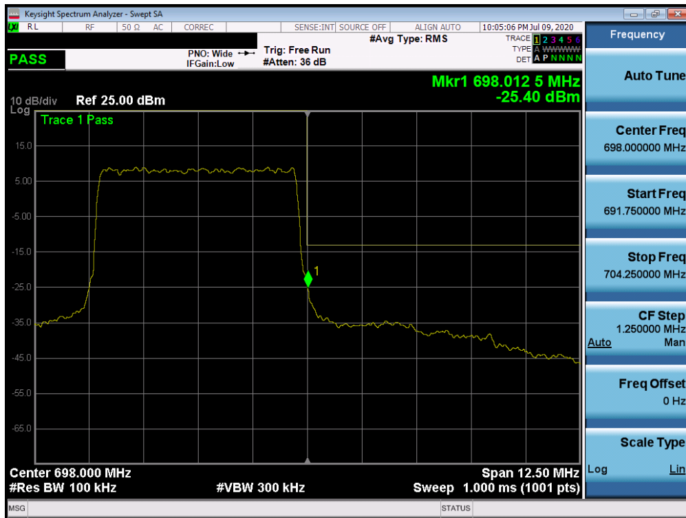
Plot 7-383. Upper Band Edge Plot (n71 - 5MHz DFT-s-OFDM-QPSK - Full RB Configuration)
