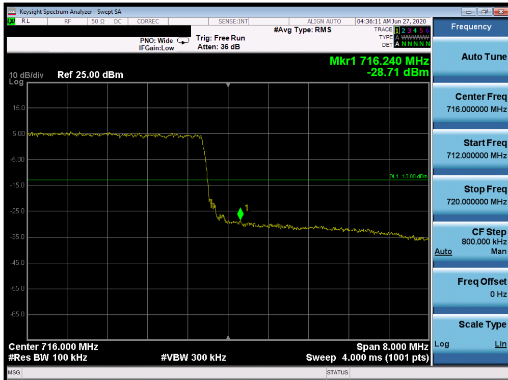
Plot 7-399. Upper Band Edge Plot (Band 12/17 - 10.0MHz QPSK - Full RB Configuration)
