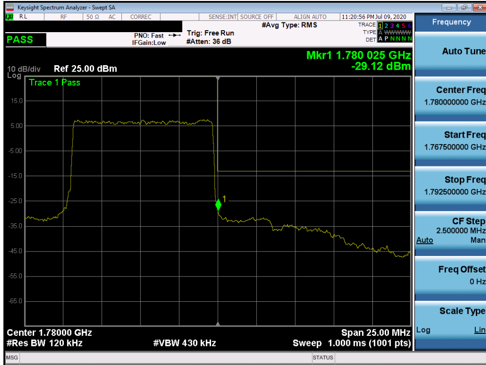
Plot 7-454. Upper Band Edge Plot (n66 - 10MHz DFT-s-OFDM-QPSK - Full RB Configuration)
