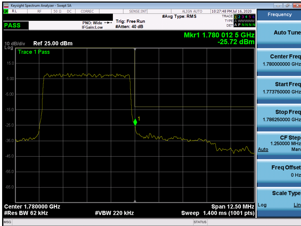
Plot 7-470. Upper Band Edge Plot (n66 - 5MHz DFT-s-OFDM-QPSK - Full RB Configuration)
