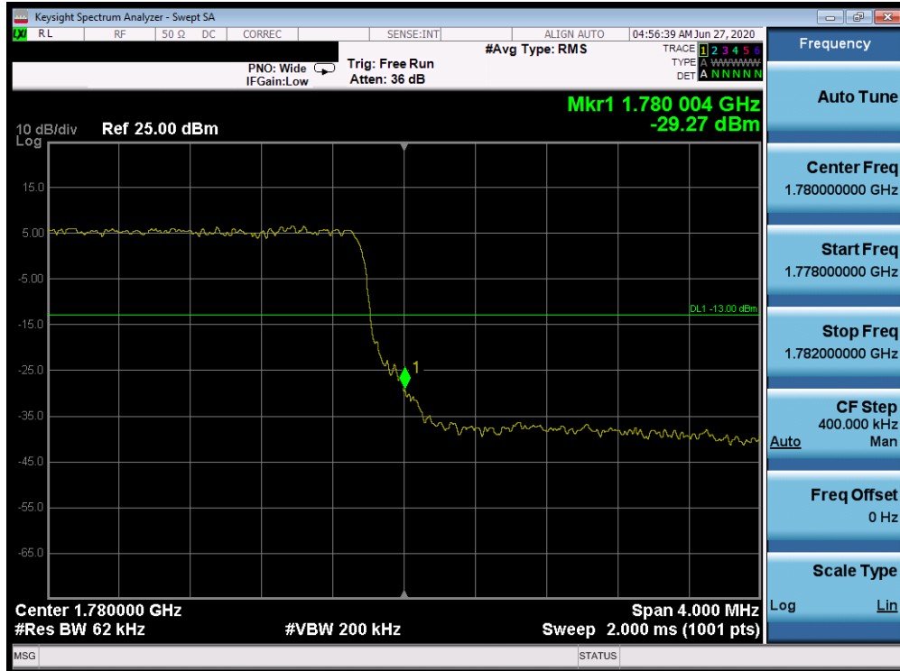
Plot 7-428. Upper Band Edge Plot (Band 66 - 5.0MHz QPSK - Full RB Configuration)
