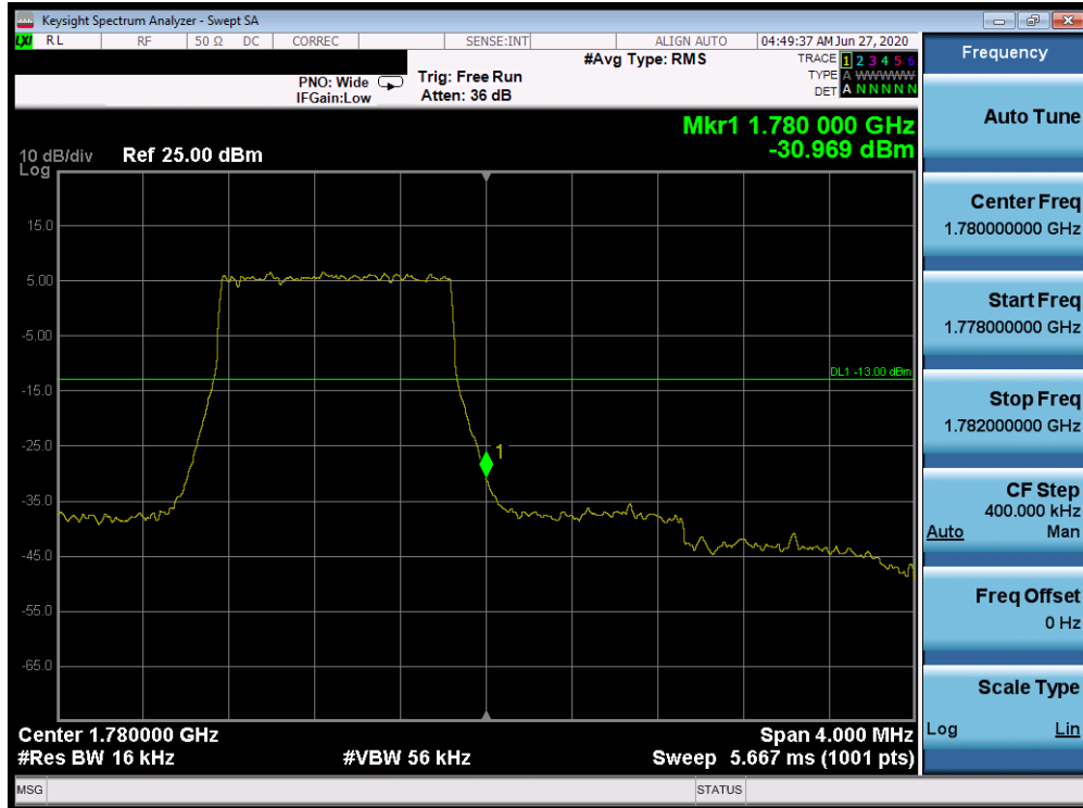
Plot 7-416. Upper Band Edge Plot (Band 66 - 1.4MHz QPSK - Full RB Configuration)
