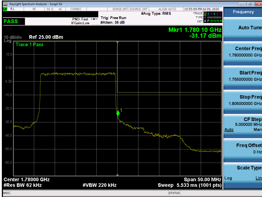
Plot 7-462. Upper Band Edge Plot (n66 - 20MHz DFT-s-OFDM-QPSK - Full RB Configuration)
