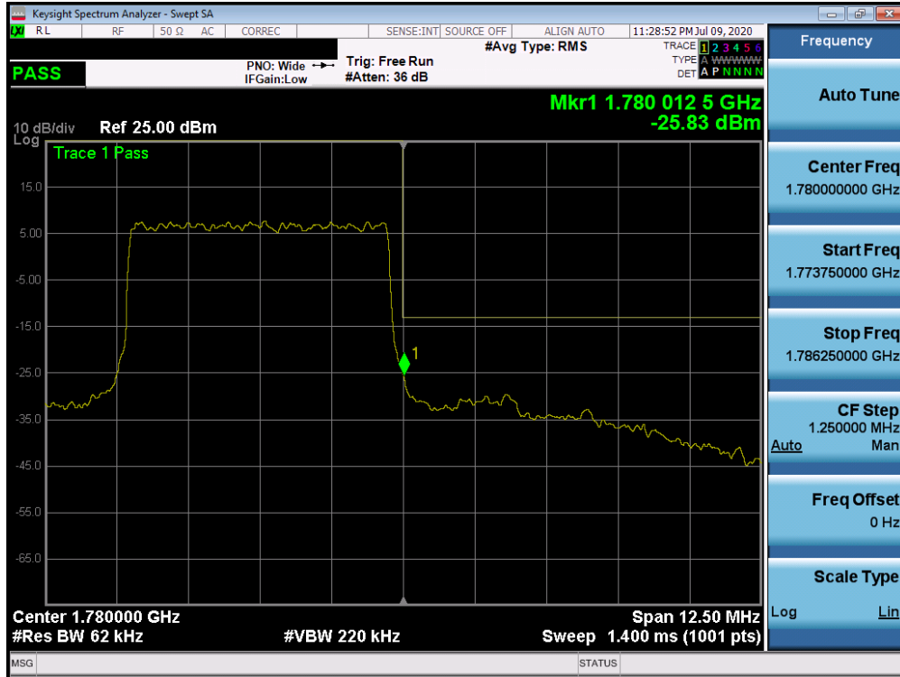
Plot 7-450. Upper Band Edge Plot (n66 - 5MHz DFT-s-OFDM-QPSK - Full RB Configuration)
