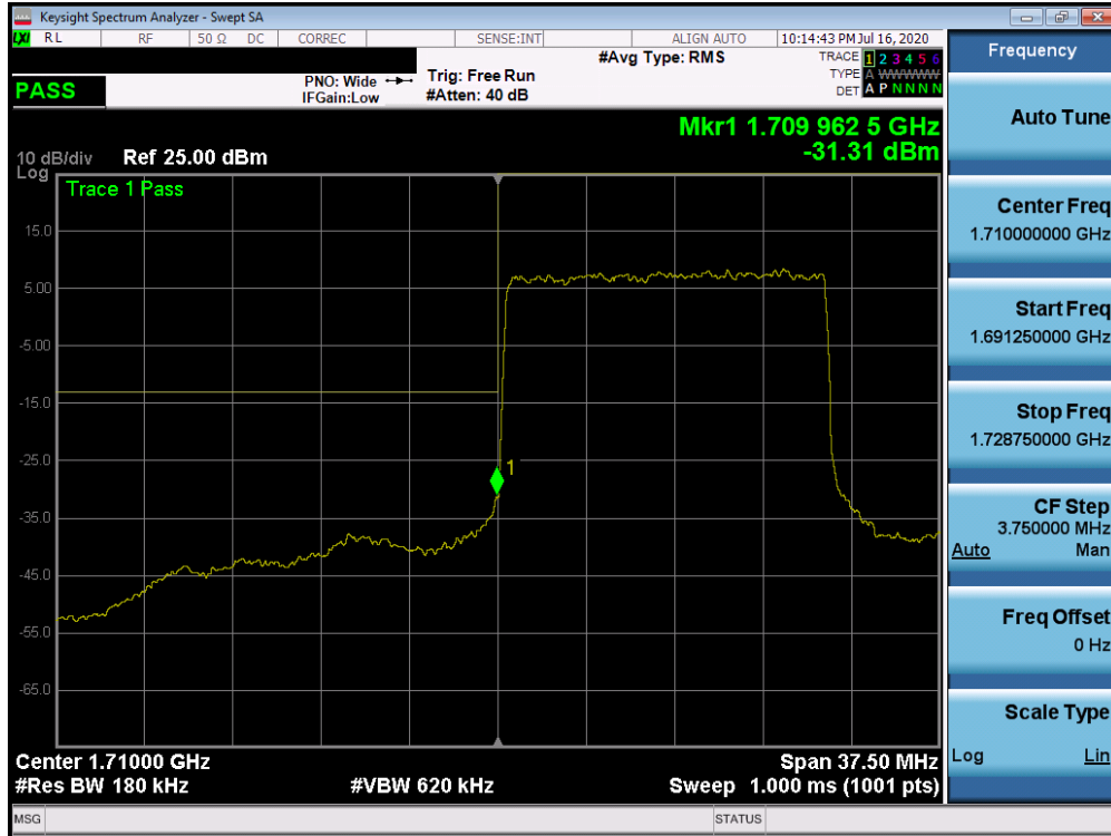
Plot 7-476. Lower Band Edge Plot (n66 - 15MHz DFT-s-OFDM-QPSK - Full RB Configuration)
