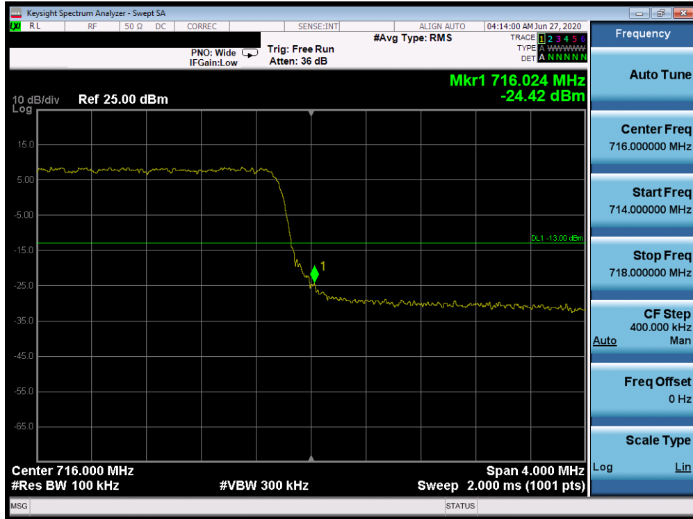
Plot 7-396. Upper Band Edge Plot (Band 12/17 - 5.0MHz QPSK - Full RB Configuration)
