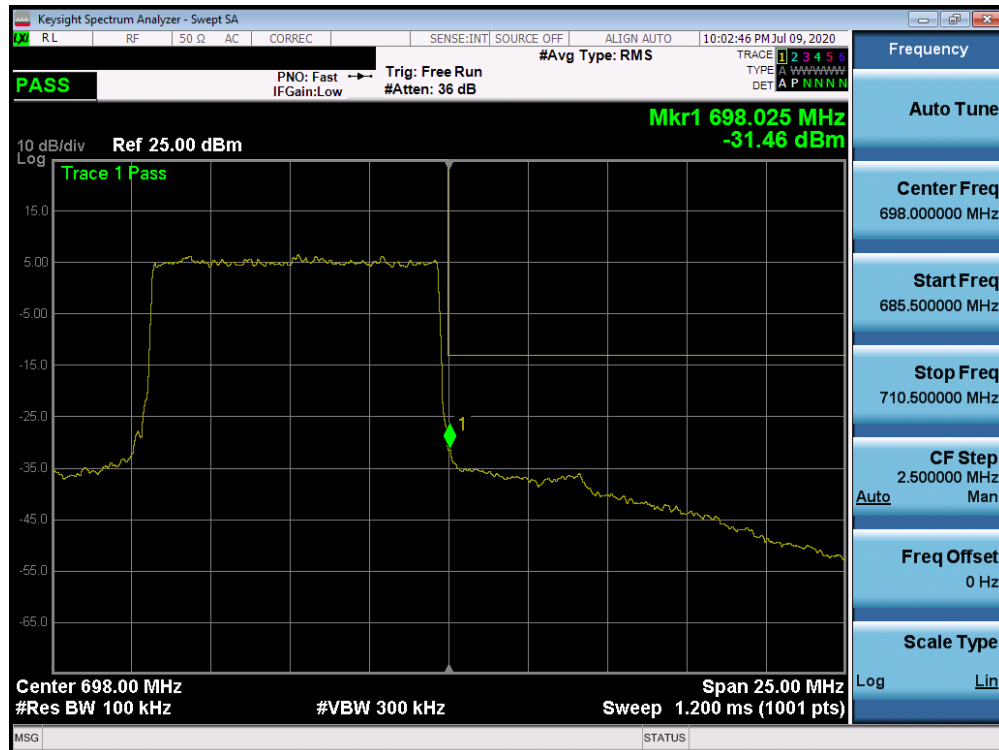
Plot 7-385. Upper Band Edge Plot (n71 - 10MHz DFT-s-OFDM-QPSK - Full RB Configuration)
