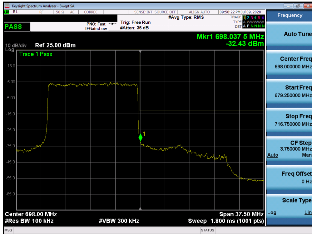
Plot 7-387. Upper Band Edge Plot (n71 - 15MHz DFT-s-OFDM-QPSK - Full RB Configuration)
