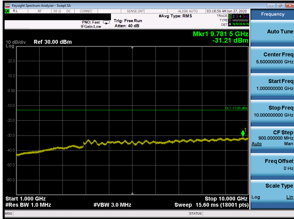
Plot 7-301. Conducted Spurious Plot (Band 26 - 15.0MHz QPSK - RB Size 1, RB Offset 0 - High Channel)
