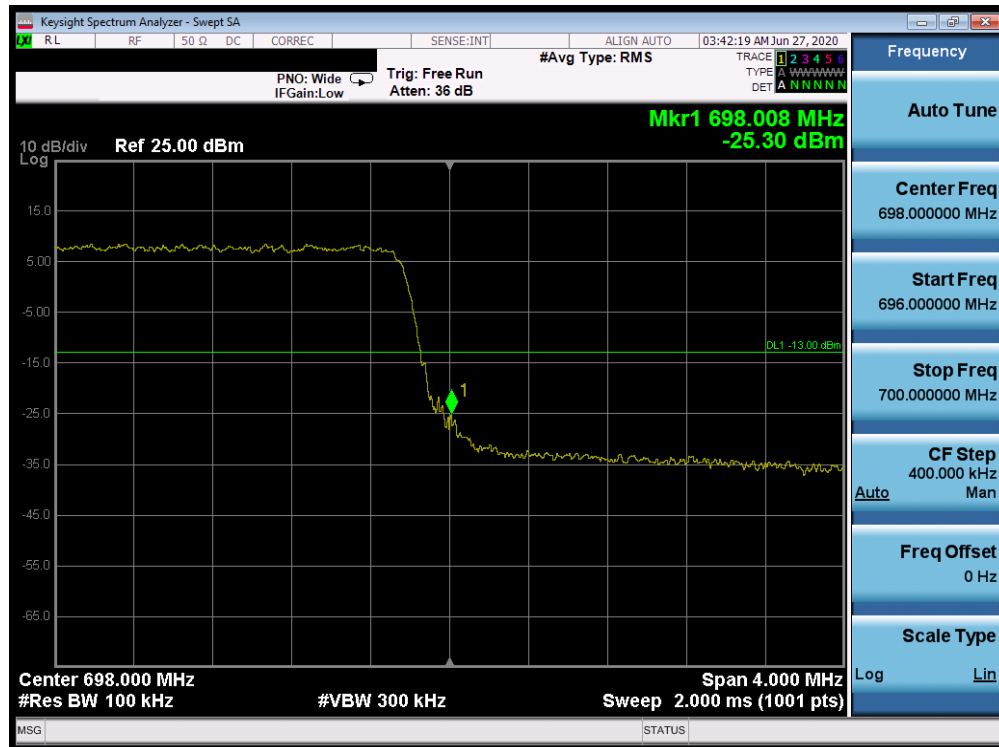
Plot 7-375. Upper Band Edge Plot (Band 71 - 5.0MHz QPSK - Full RB Configuration)
