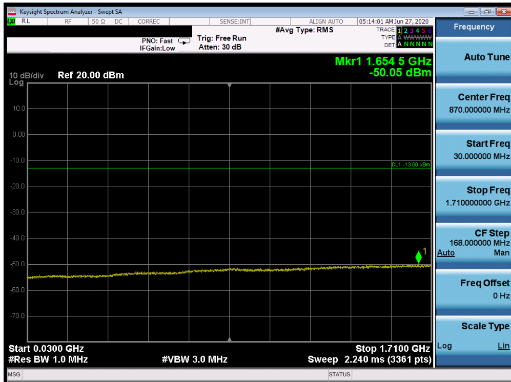
Plot 7-305. Conducted Spurious Plot (Band 66/4 - 20.0MHz QPSK - RB Size 1, RB Offset 0 - Mid Channel)
