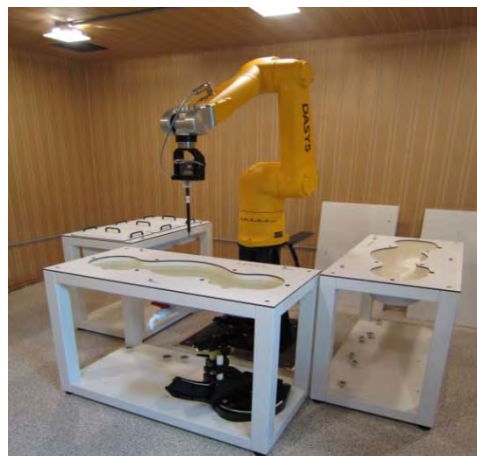
Figure E.7.1 DASY5 Test System
