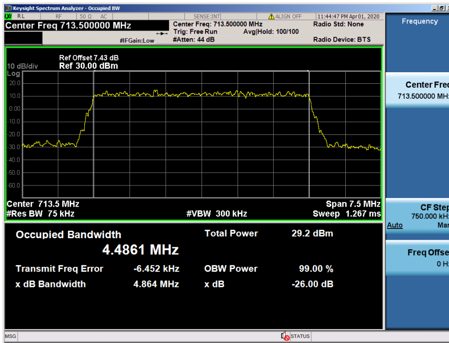
LTE Band 12, 17 / 5 MHz / 64QAM - RB Size 25
