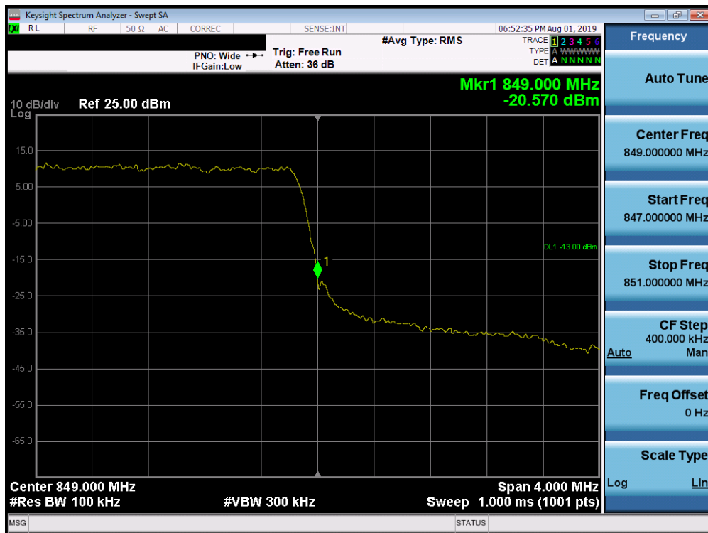
Plot 7-206. Upper Band Edge Plot (Band 26/5 - 3.0MHz QPSK - Full RB Configuration)
