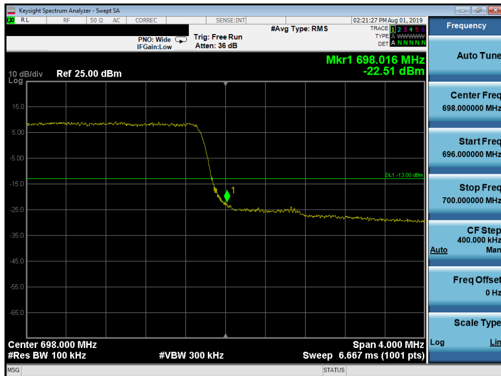
Plot 7-182. Upper Band Edge Plot (Band 71 - 5.0MHz QPSK - Full RB Configuration)
