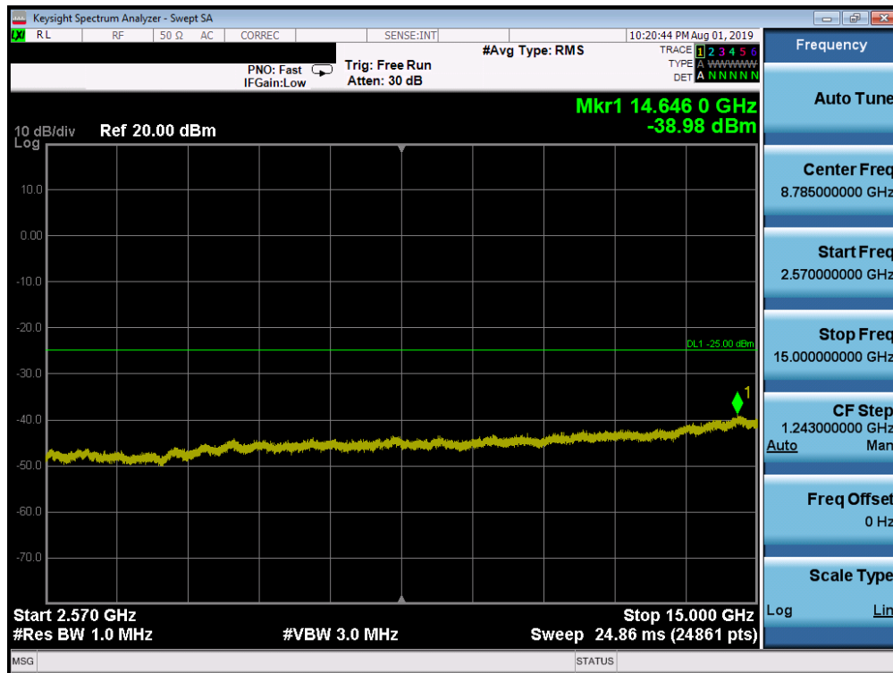
Plot 7-164. Conducted Spurious Plot (Band 7 - 20.0MHz QPSK - RB Size 1, RB Offset 0 - Low Channel)
