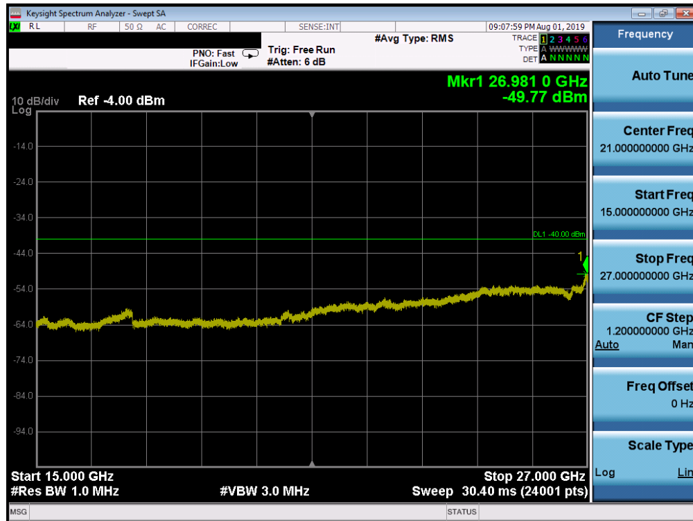
Plot 7-162. Conducted Spurious Plot (Band 30 - 10.0MHz QPSK - RB Size 1, RB Offset 0 – Mid Channel)
