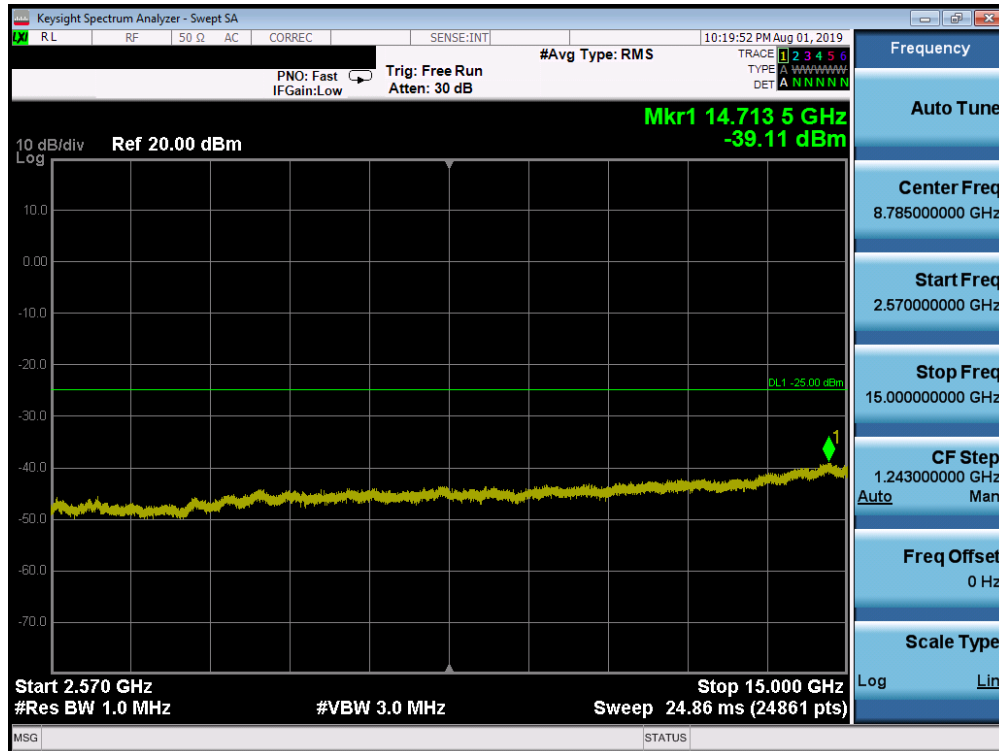
Plot 7-167. Conducted Spurious Plot (Band 7 - 20.0MHz QPSK - RB Size 1, RB Offset 0 – Mid Channel)
