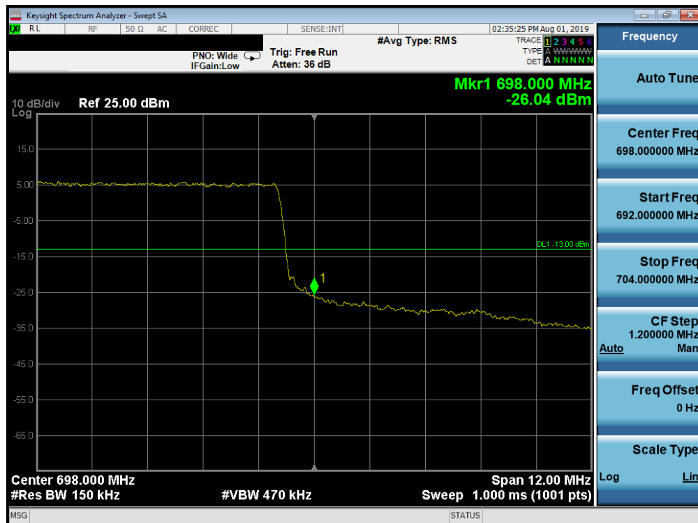
Plot 7-186. Upper Band Edge Plot (Band 71 - 15.0MHz QPSK - Full RB Configuration)
