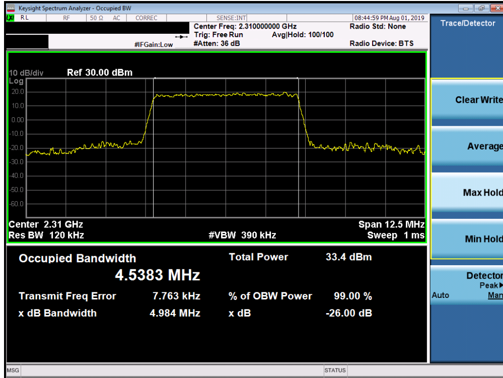
Plot 7-82. Occupied Bandwidth Plot (Band 30 – 5.0MHz QPSK - Full RB Configuration)
