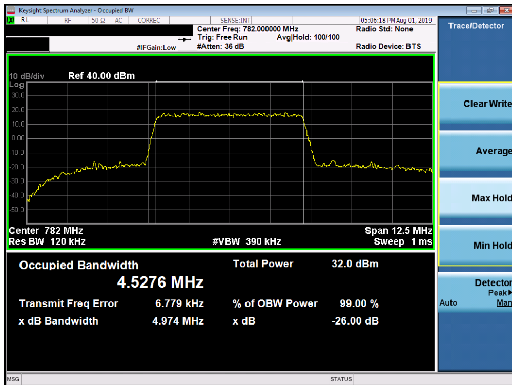
Plot 7-26. Occupied Bandwidth Plot (Band 13 – 5.0MHz 16-QAM – Full RB Configuration)
