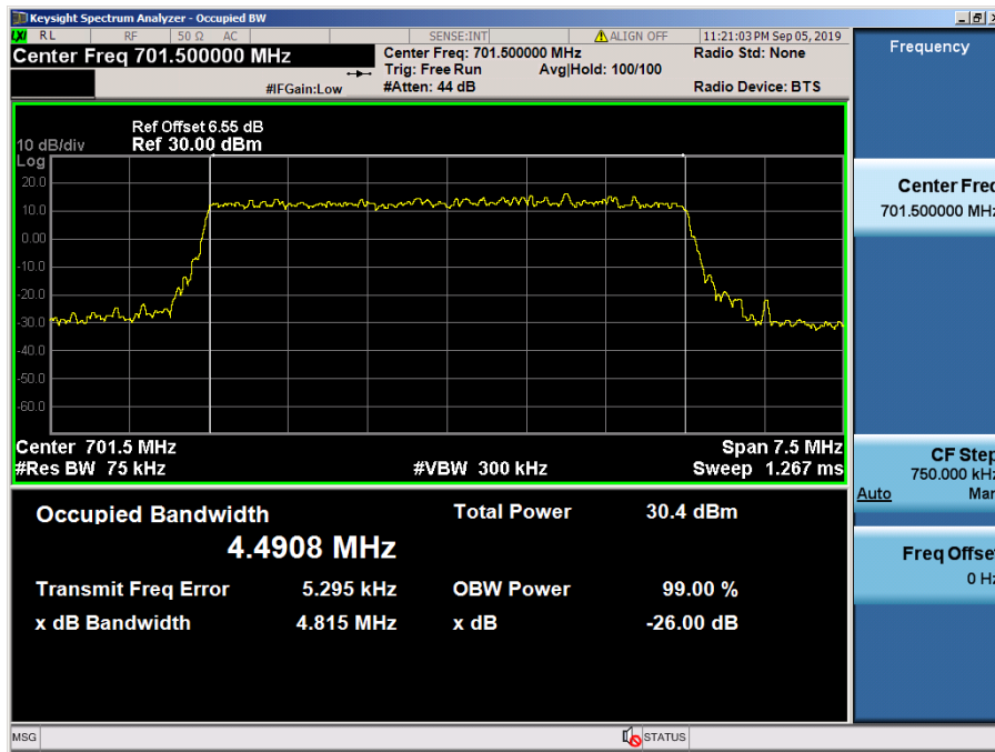
LTE Band 12, 17 / 5 MHz / 64QAM - RB Size 25
